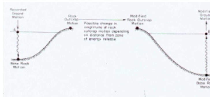
Fig. 4. Schematic representation of procedure for computing effects of local soil conditions on ground motions (after Schnabel et al., 1971)
