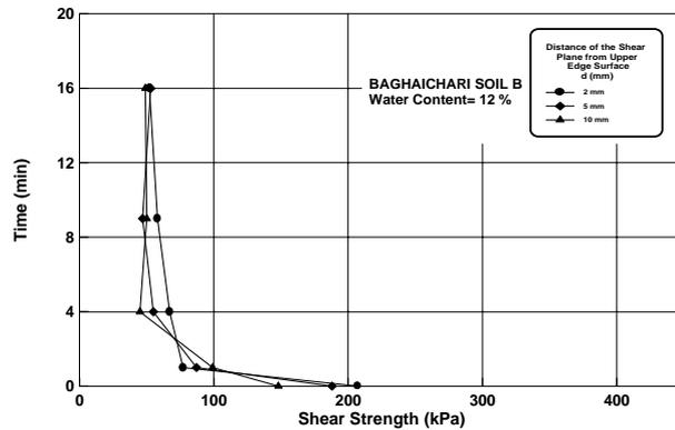
Fig 2b. Variation of Shear Strength with Water Supply Duration (Baghaichari Soil B)
