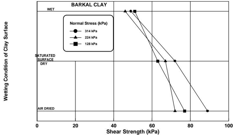
Fig 4. Variation of Shear Strength at Various Wetting Conditions of Clay Surface (Barkal Clay)
