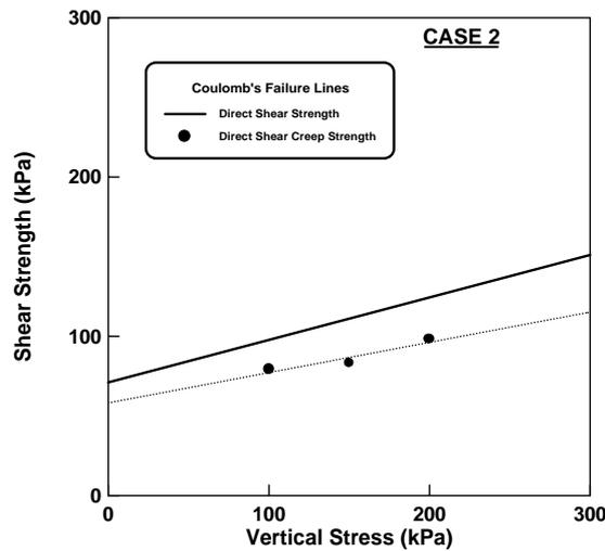
Fig 6a. Creep Shear Strength Test Showing Coulomb's Failure Line (Case 2)
