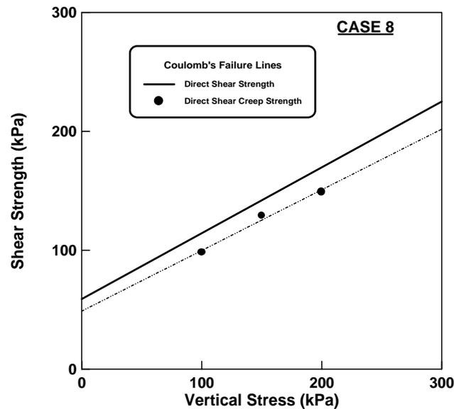
Fig 6c. Creep Shear Strength Test Showing Coulomb's Failure Lines (Case 8)
