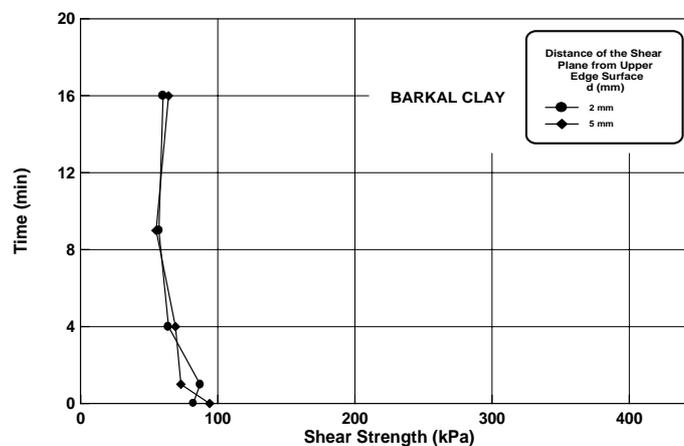
Fig 3. Relationship between Shear Strength with Water Supply Duration (Barkal Clay)
