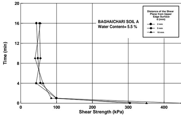
Fig 2a. Variation of Shear Strength with Water Supply Duration Baghaichari Soil A)
