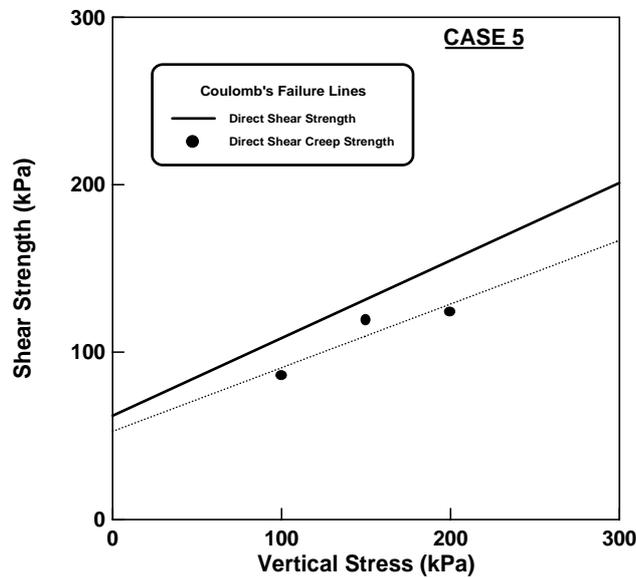
Fig 6b. Creep Shear Strength Test Showing Coulomb's Failure Lines (Case 5)
