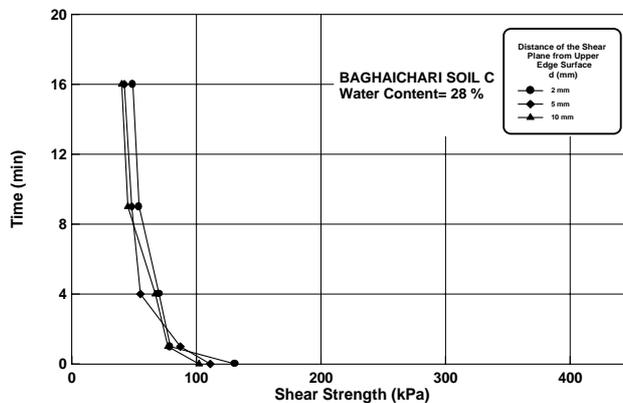
Fig 2c. Variation of Shear Strength with Water Supply Duration (Baghaichari Soil C)
