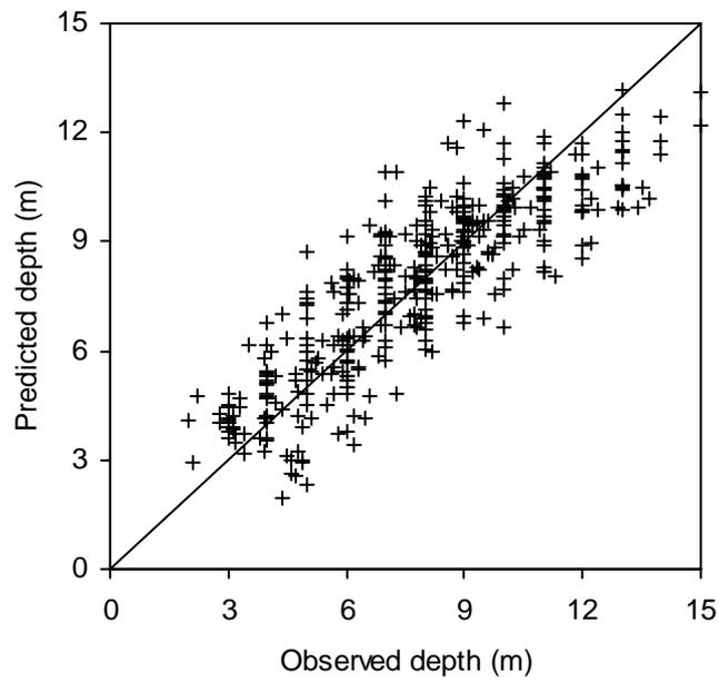
Fig. 2. Comparison of the observed and predicted flow depth after applying the correction factor
