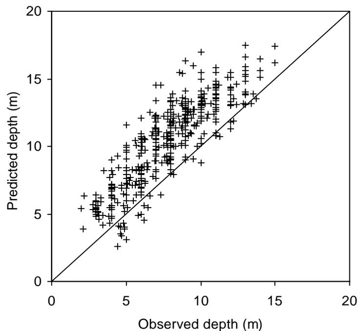
Fig. 1. Comparison of the observed and predicted flow depth
