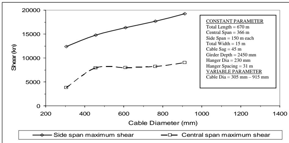
Fig. 12. Variation of central and side span maximum shear with cable diameter
