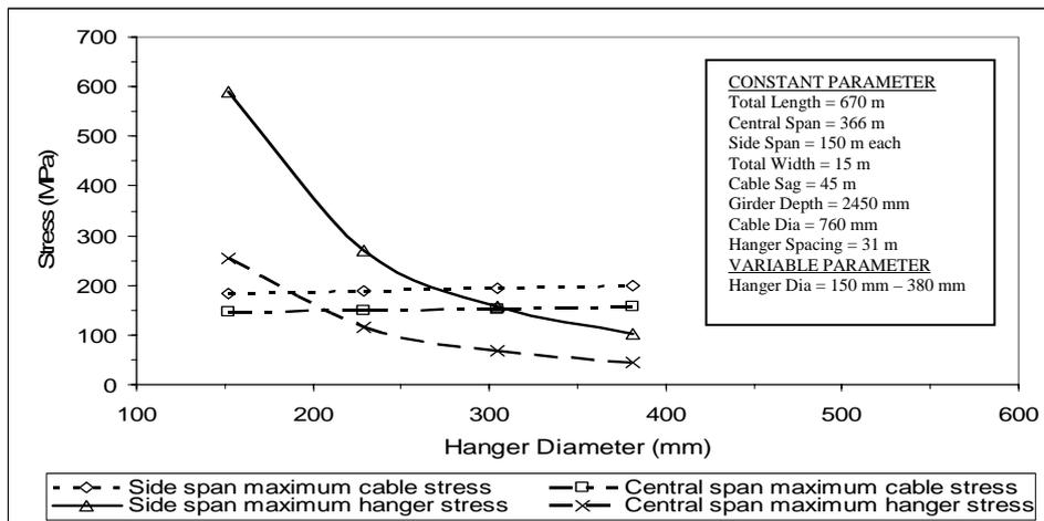
Fig. 15. Variation of central and side span maximum cable and hanger stress with hanger diameter
