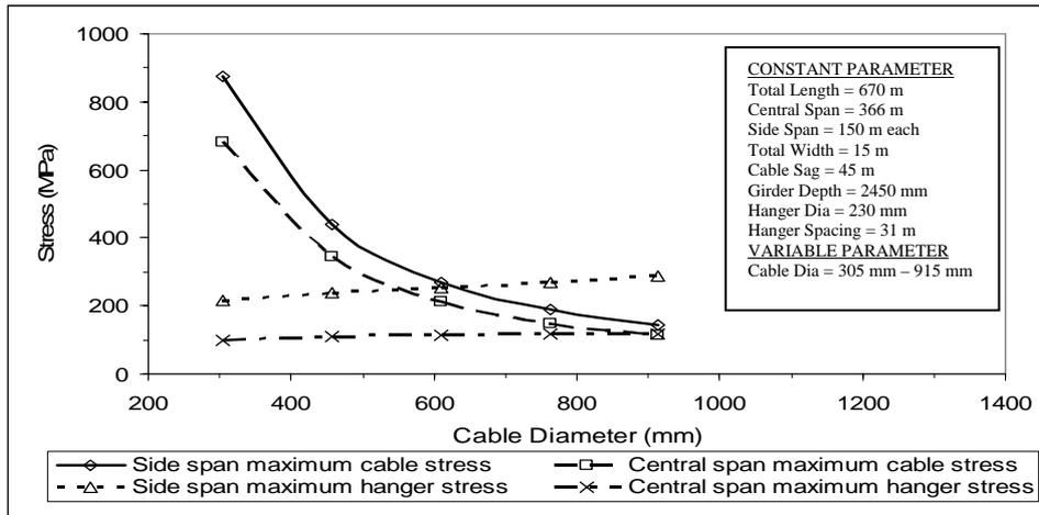
Fig. 11. Variation of central and side span maximum cable and hanger stress with cable diameter
