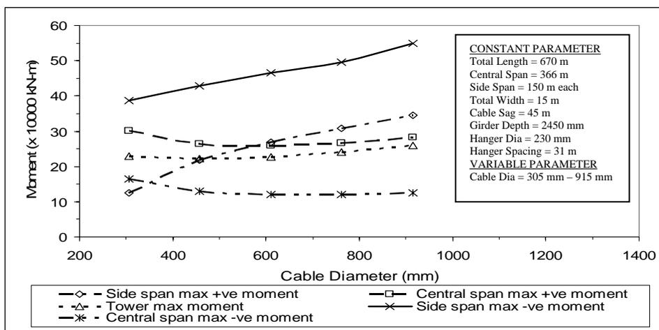
Fig. 10. Variation of maximum tower, central and side span maximum moments with cable diameter
