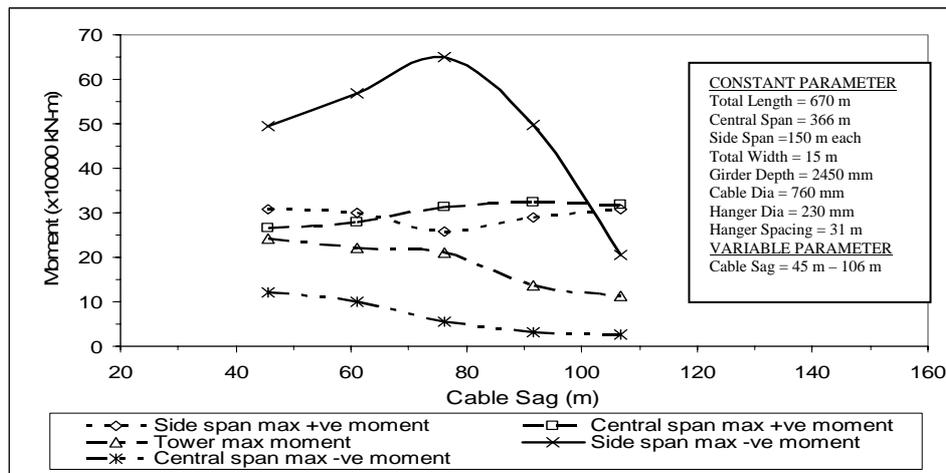
Fig. 2. Variation of maximum tower, central and side span maximum moments with cable sag
