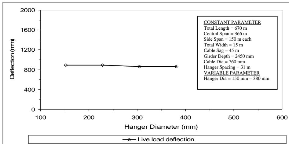
Fig. 17. Variation of maximum live load deflection with hanger diameter
