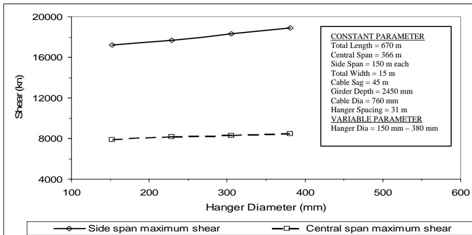
Fig. 16. Variation of central and side span maximum shear with hanger diameter
