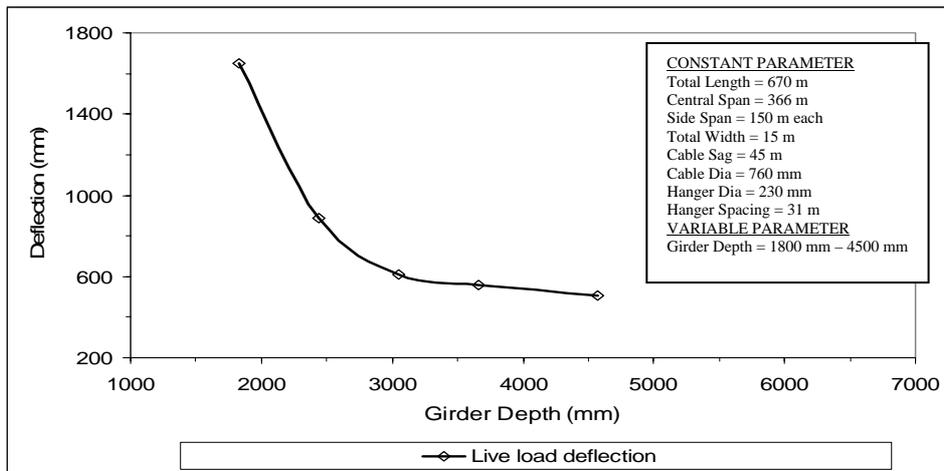
Fig. 9. Variation of maximum live load deflection with girder depth
