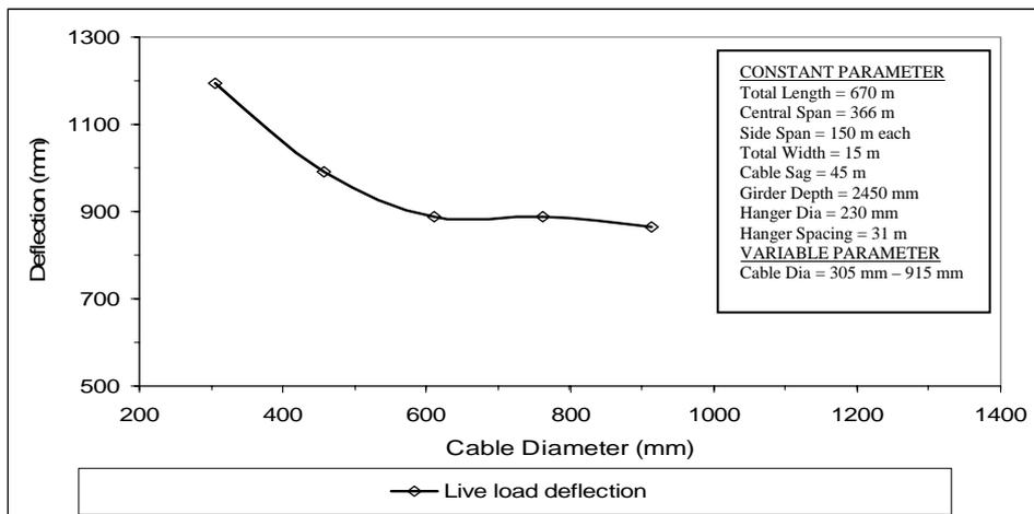
Fig. 13. Variation of maximum live load deflection with cable diameter
