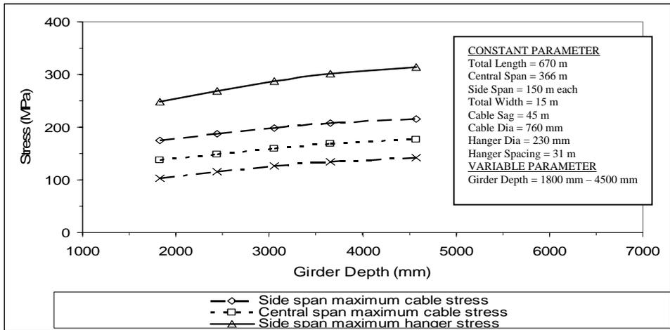
Fig. 7. Variation of central and side span maximum cable and hanger stress with girder depth
