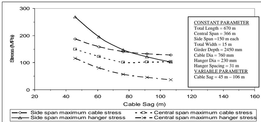
Fig. 3. Variation of central and side span maximum cable and hanger stress with cable sag
