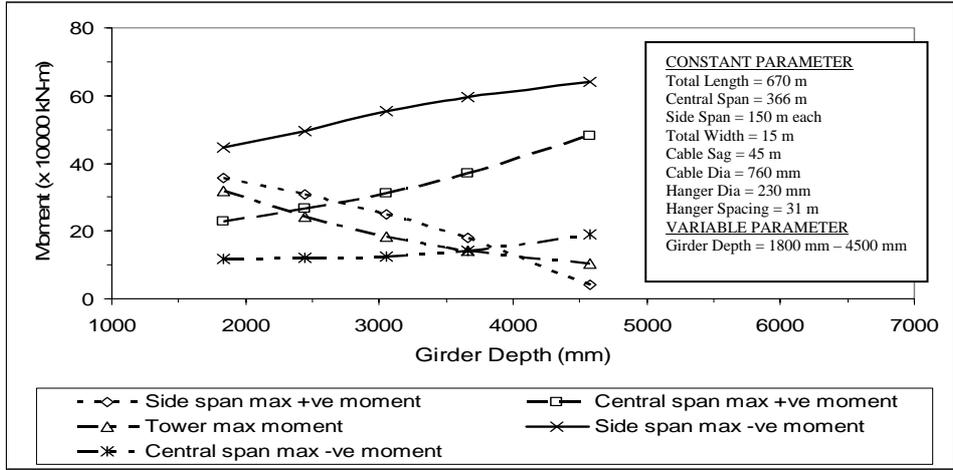
Fig. 6. Variation of maximum tower, central and side span maximum moments with girder depth
