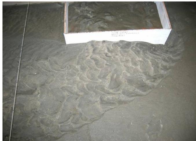
Fig. 3. Scour around vertical structure, b=60cm
