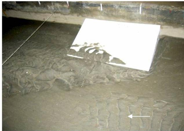
Fig. 2. Scour around the 1V:3H slope Structure
