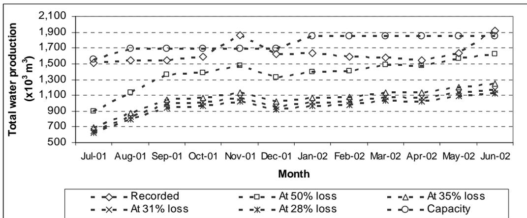
Fig. 3. Recorded and optimum water production during July/01-June/02
