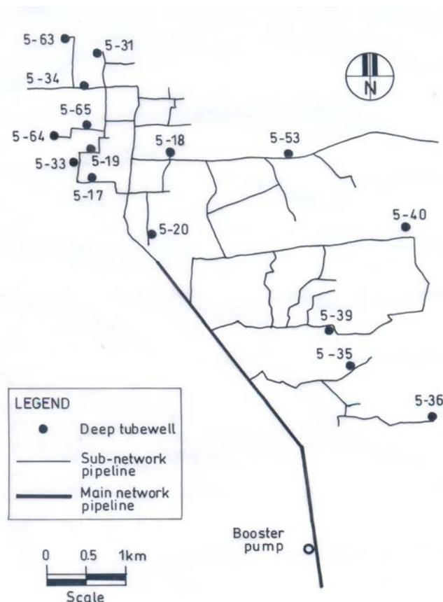
Fig. 1. Uttara water supply sub-network and deep tube well locations
