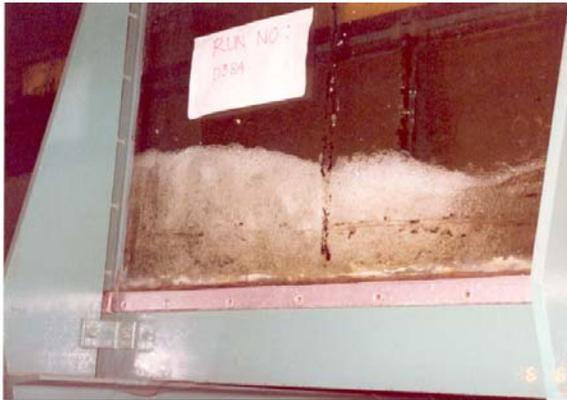
Fig. 7. Side view of a T – jump ( $B = 0.5$ , Slope =  $0.0131$ , Gate opening =  $13\text{cm}$ )
