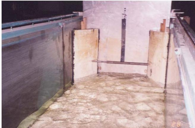
Fig. 5. Photograph of transition elements at upstream of sluice gate
