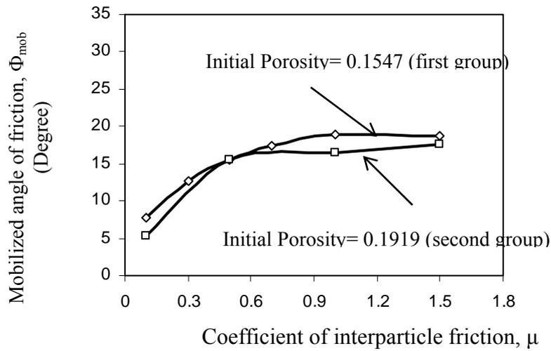
Fig. 5. Comparison of mobilized angle of friction at residual state due to the variation of initial porosity
