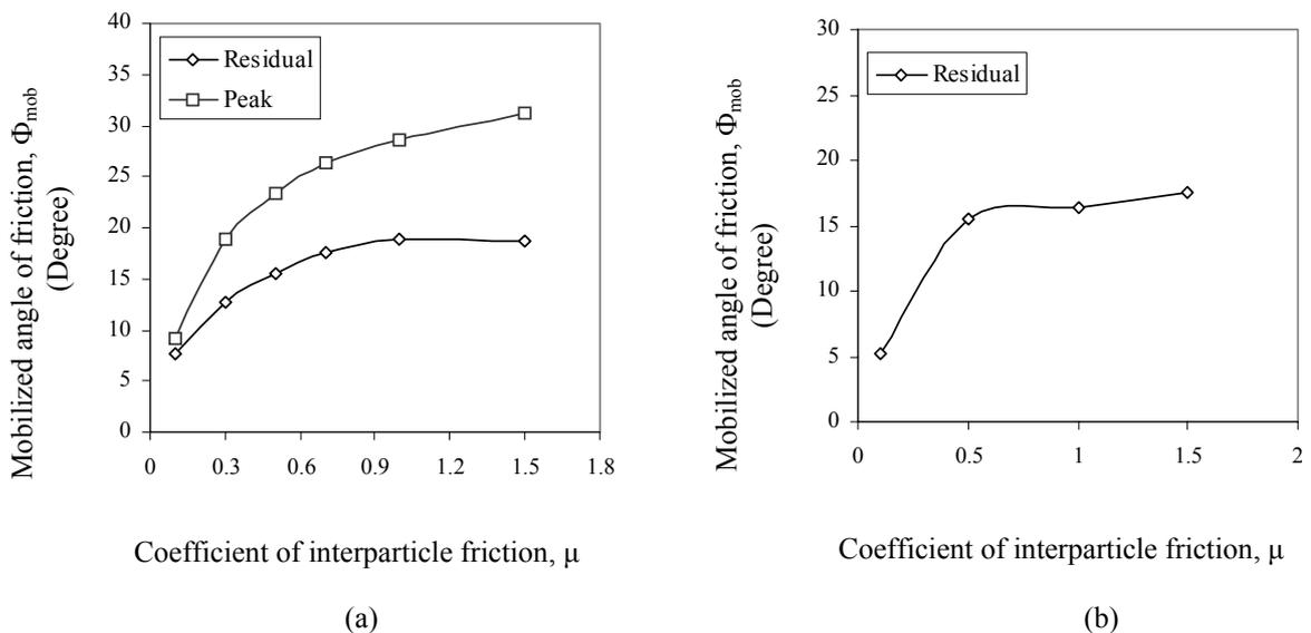
Fig. 4. Influence of the variation of interparticle friction on the mobilized angle of friction (a) For dense assemblies (first group); (b) For relatively loose assemblies (second group)
