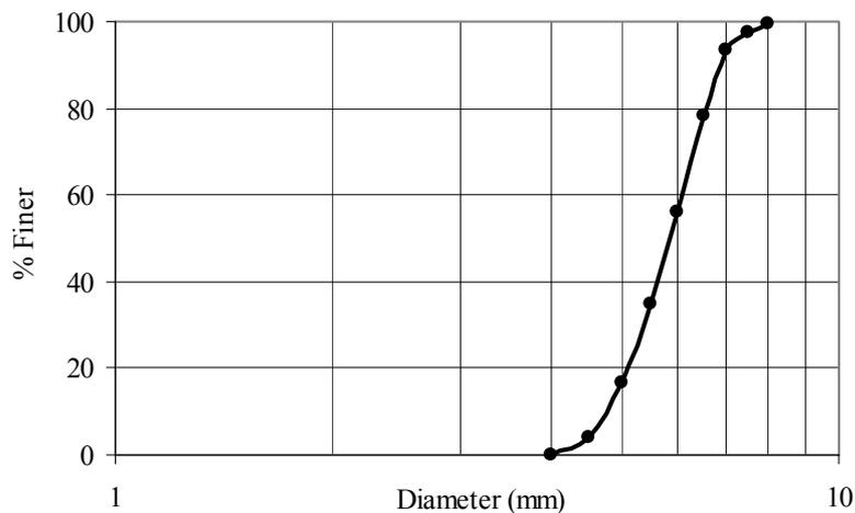
Fig. 1. Grain size distribution of circular particles used in the simulation
