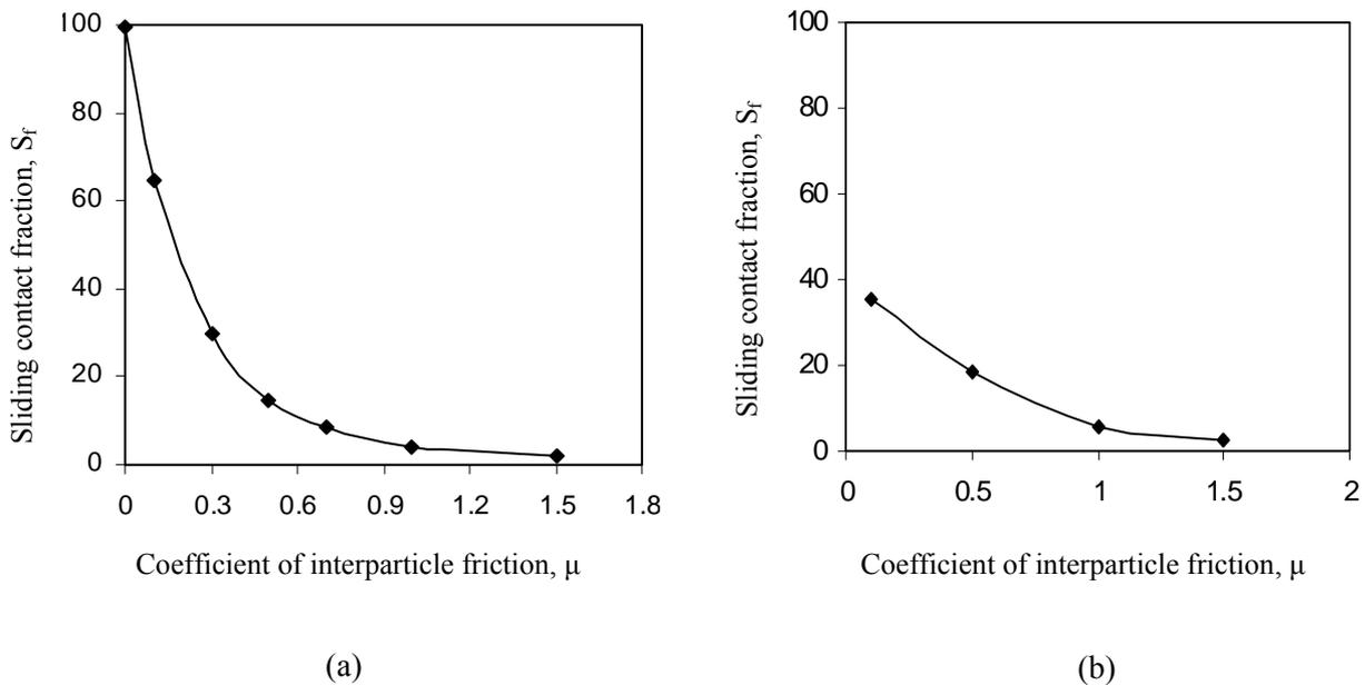
Fig. 6. Influence of the variation of interparticle friction on sliding contact fraction at residual state in (a) dense system; (b) relatively loose system
