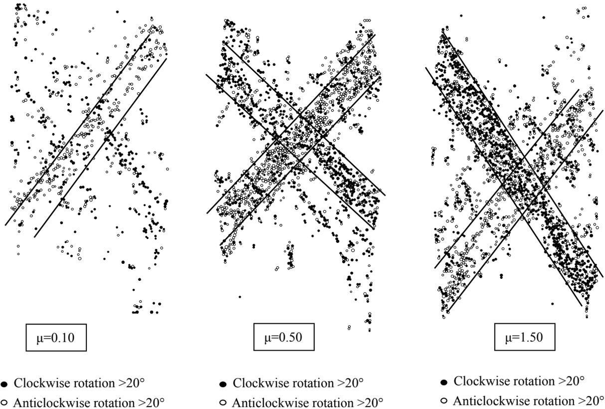
Fig. 7. Influence of the variation of interparticle friction on the distribution of highly rotated particles in dense granular system (first group).
