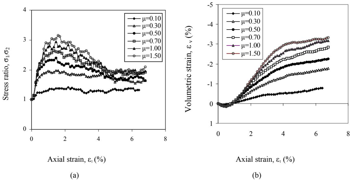
Fig. 3. (a) Stress-strain response; (b) volumetric strain response of dense granular assembly (first group) under various interparticle friction coefficients
