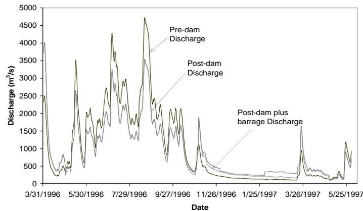
Figure 5 Boundary discharge of the Barak at Amalshid point for the average year pre- dam, post-dam and barrage, and only post-dam.
