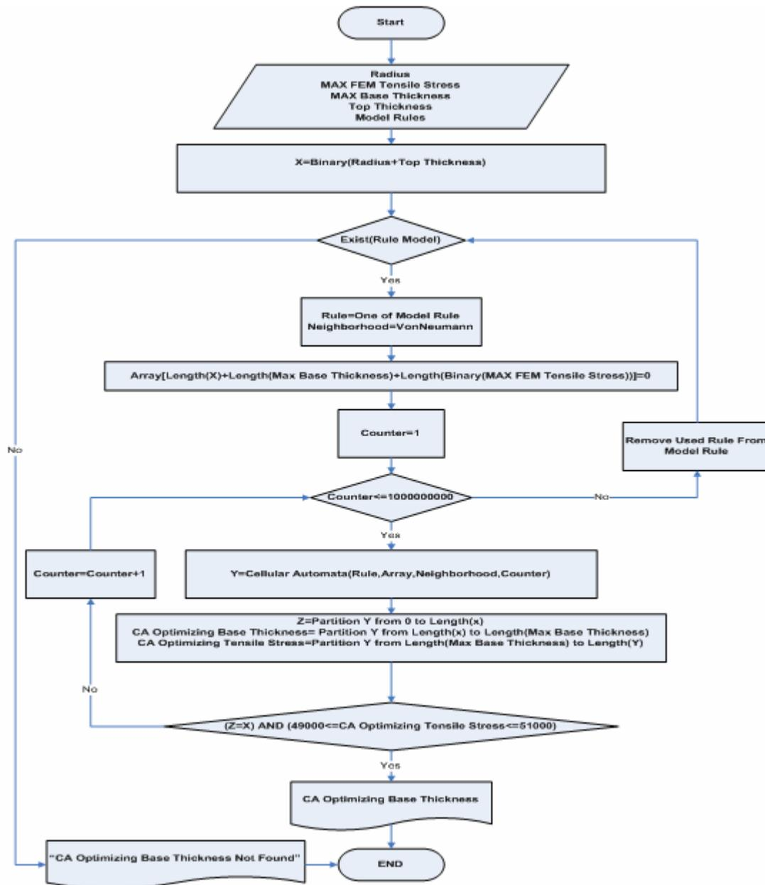
Fig. 12. Algorithm of arch thickness optimization using two -state -1-D cellular automata
