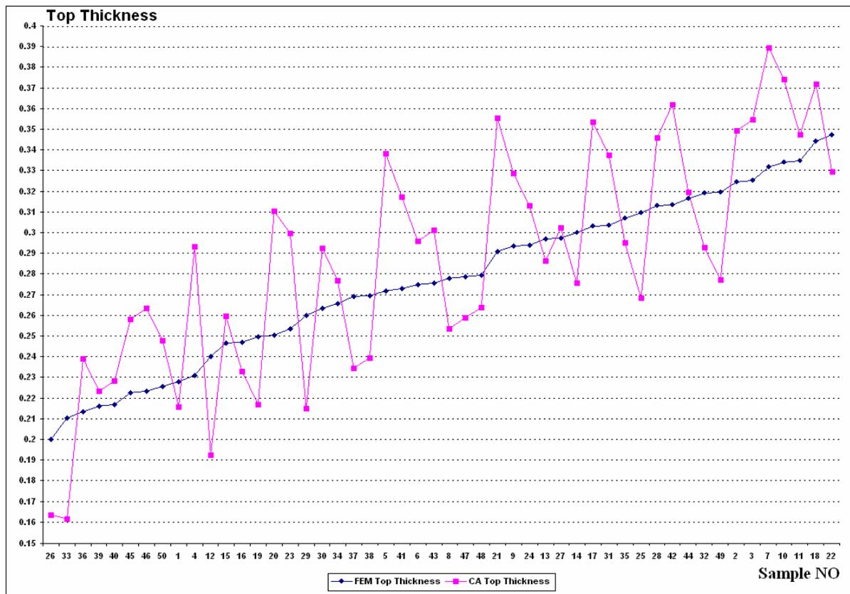
Fig. 15. Comparison of optimum range of arch top thickness using CA model and FEM software
