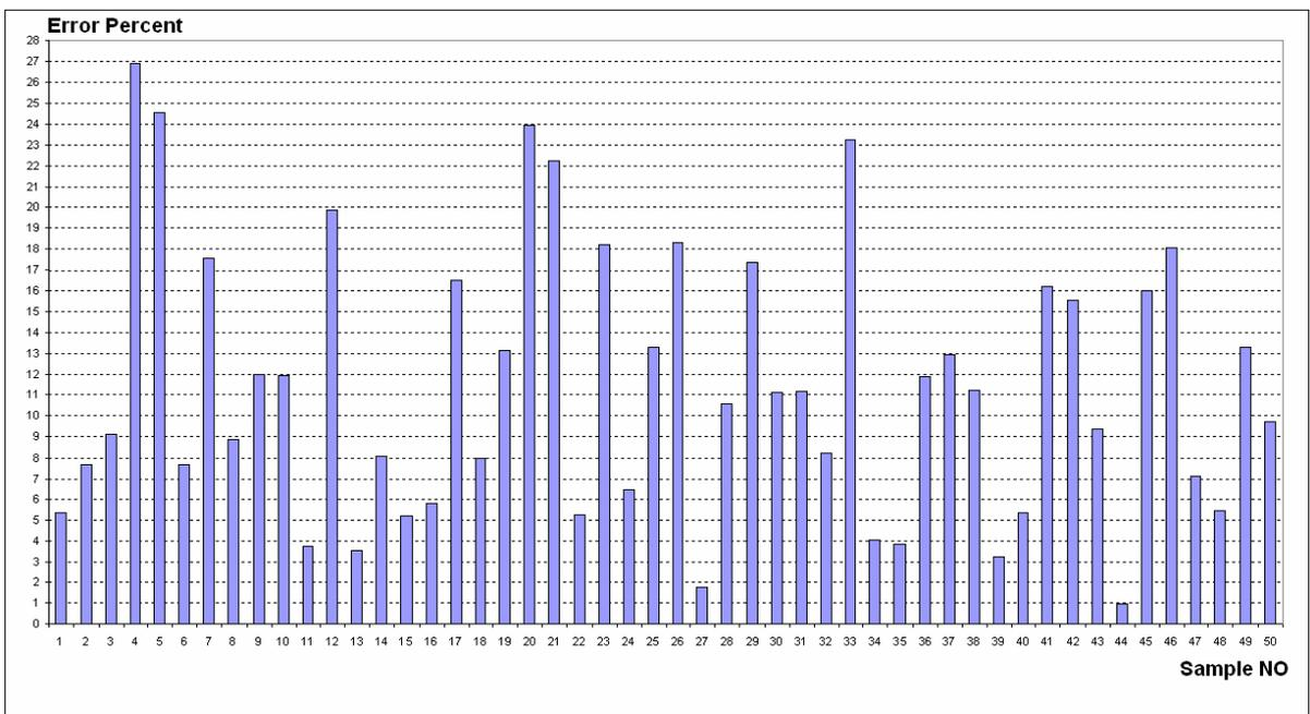
Fig. 14. Error percent of top thickness optimization in semicircular arch using CA model towards FEM software
