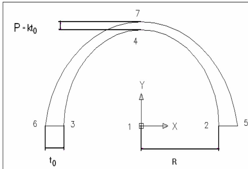
Fig. 3. Geometrical model of semicircular arch
