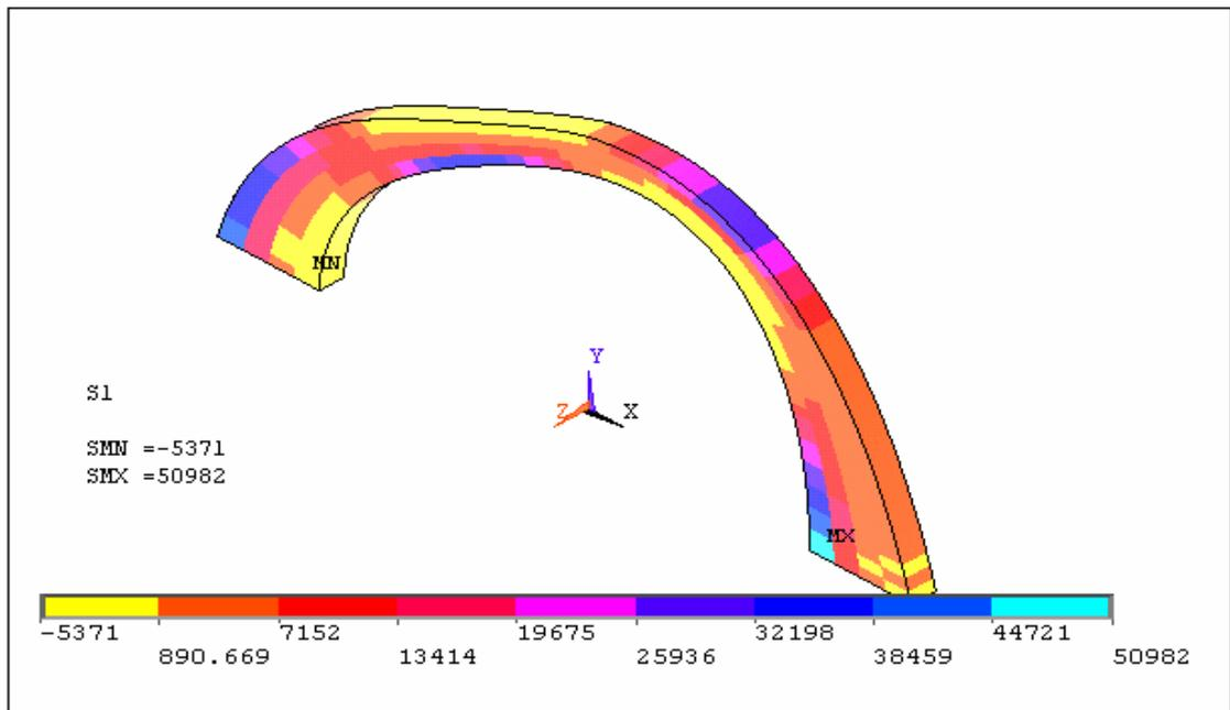
Fig. 2. Optimum shape of semicircular arch using FEM software
