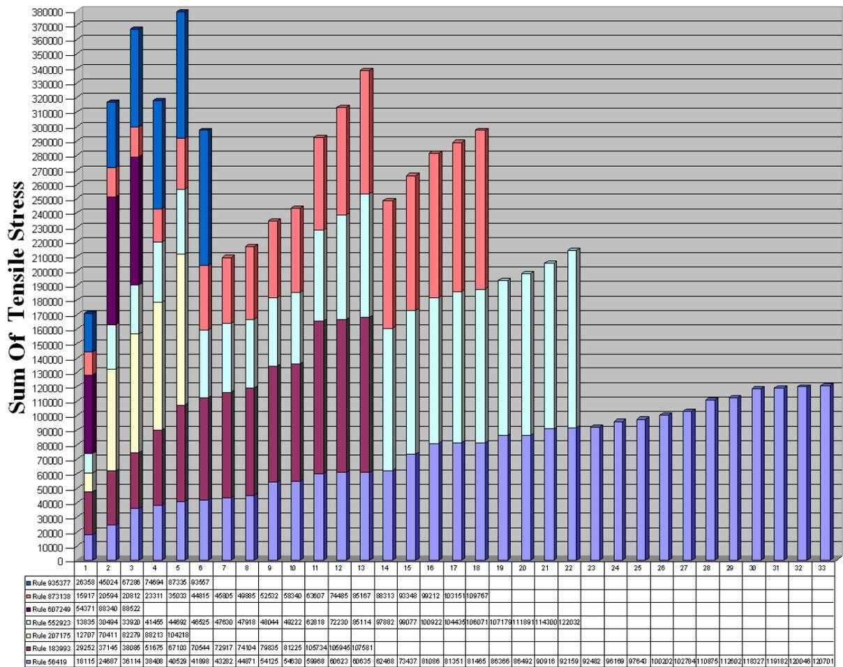
Fig. 7. Diagram of maximum tensile stress efficiency for each of cellular automata rules in semicircular arch
