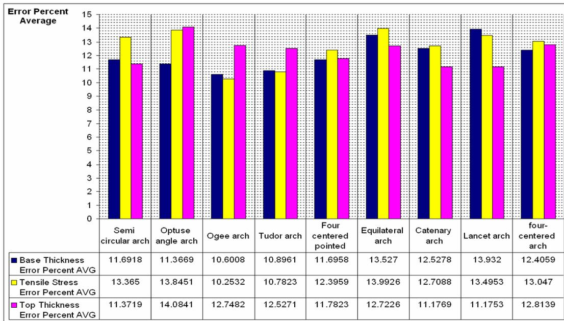
Fig. 21. Comparison between the mean of error percent of analysis of tensile stress and optimization of base and top thickness for discussed arches using CA model toward FEM software
