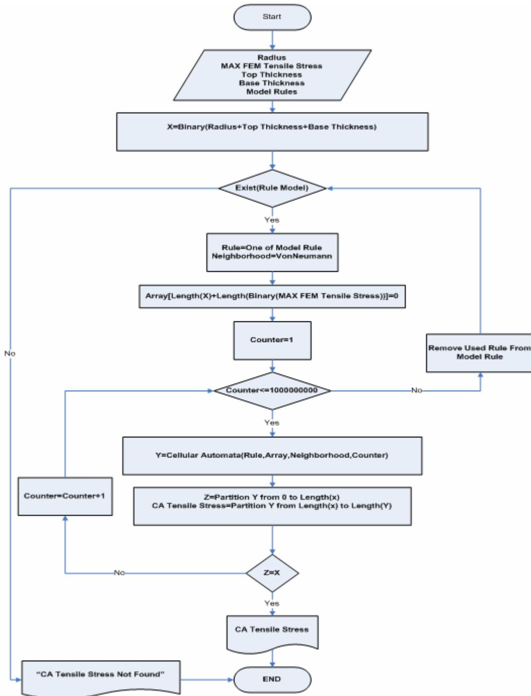
Fig. 8. An algorithm for analysis of arch behavior using two-state 1-D CA for maximum tensile stress
