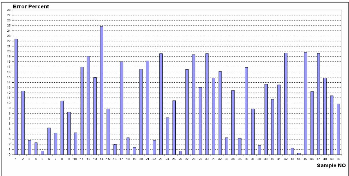
Fig. 17. Error percent of base thickness optimization in semicircular arch using CA model towards FEM software
