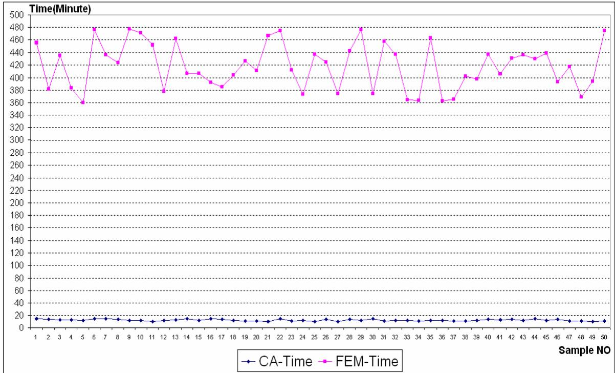
Fig. 16. Comparison between optimization time of base thickness in semicircular arch using FEM software and CA model
