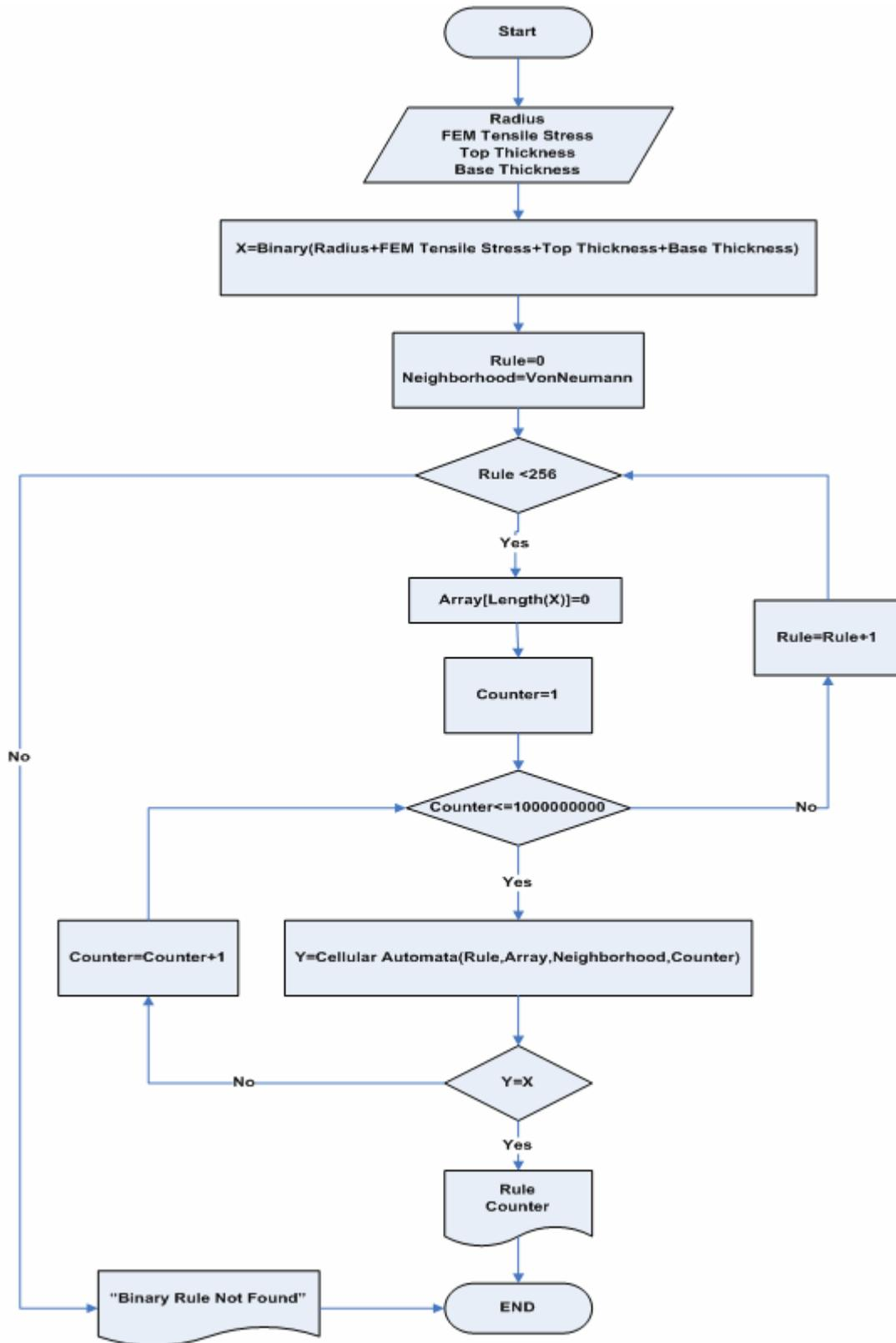
Fig. 5. An algorithm for finding two- state 1-D cellular automata model for arch behavior modeling
