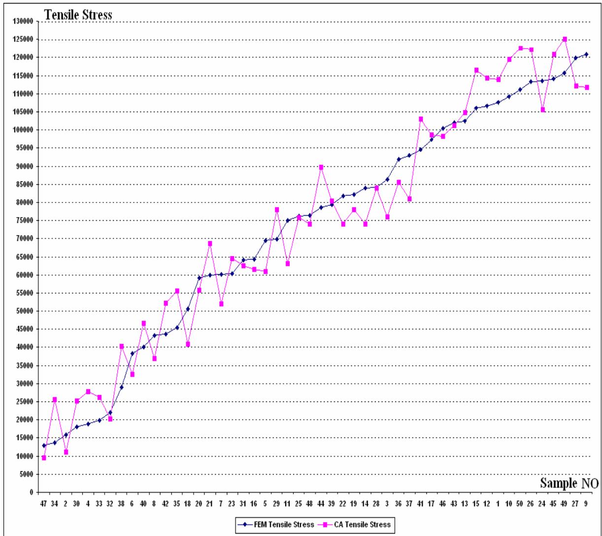
Fig.9. Comparison between maximum tensile stress using FEM software and CA model in semicircular arch
