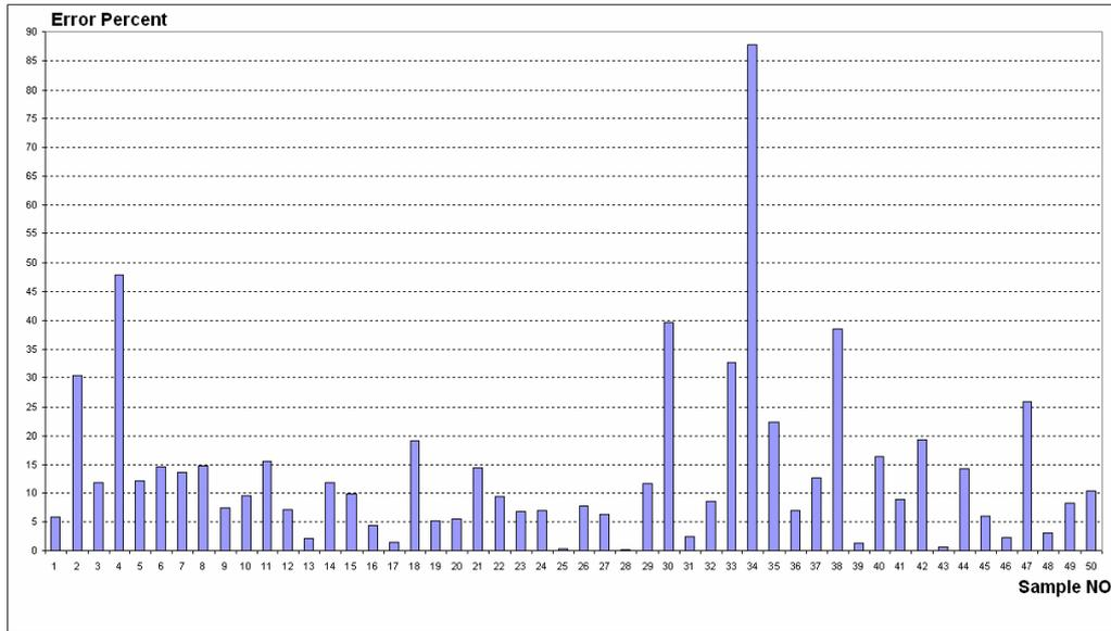
Fig. 10. Error percent of maximum tensile stress computation by CA to FEM software in semicircular arch
