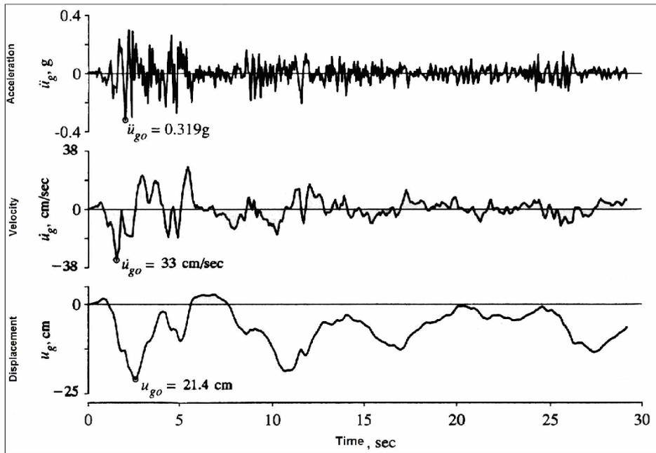
Fig. 1. North-south horizontal component of Elcentro earthquake
