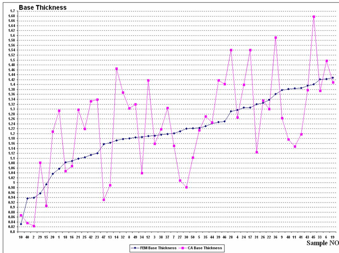
Fig. 18. Comparison of optimum range of arch base thickness using CA model and FEM software
