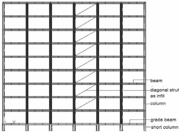
Fig.2.c FE mesh of the building in elevation with 10% infill
