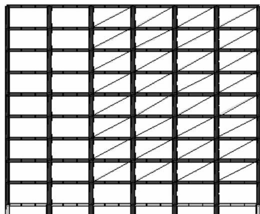
Fig.2.f FE mesh of the building in elevation with 70% infill
