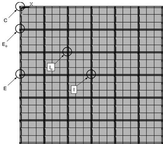
Fig.2.a FE mesh of the building in plan.
