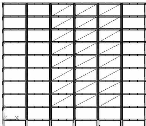
Fig.2.e FE mesh of the building in elevation with 50% infill
