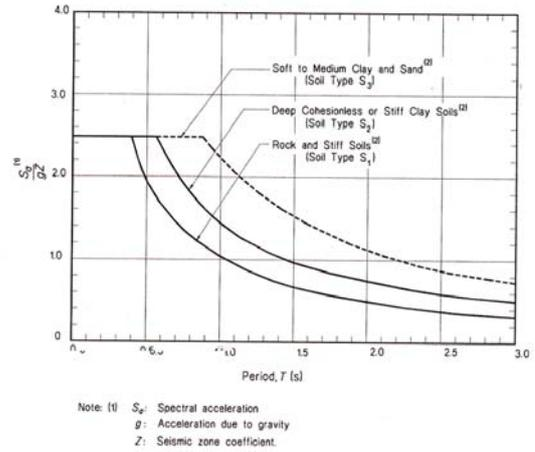
Fig.2.b Normalized Response Spectra for 5% Damping Ratio (BNBC, 2006)
