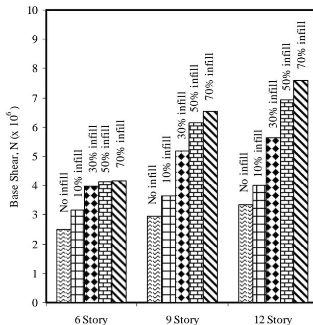
Fig. 3. Comparison of base shear for 6, 9 and 12 storied buildings for different amount of infill.
