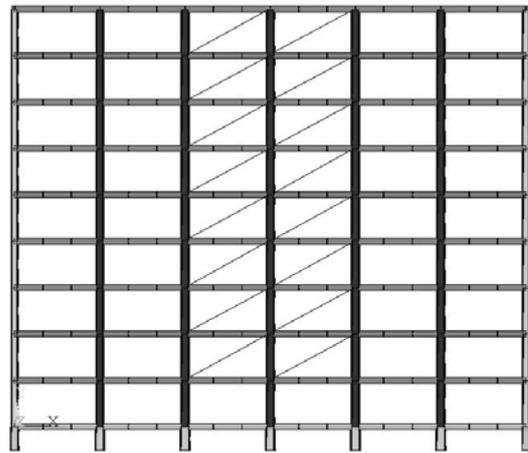
Fig.2.d FE mesh of the building in elevation with 30% infill
