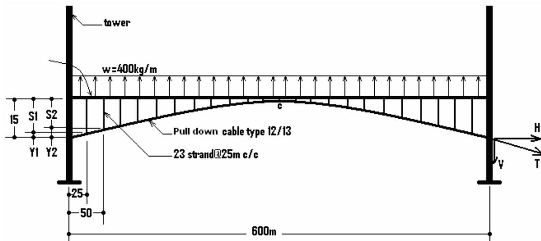
Fig. 6 Detail of a Pull-down cable system for stiffening a suspension bridge.
