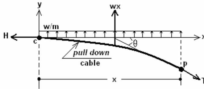
Fig. 5 Forces acting on a portion of a Pull-down cable.
