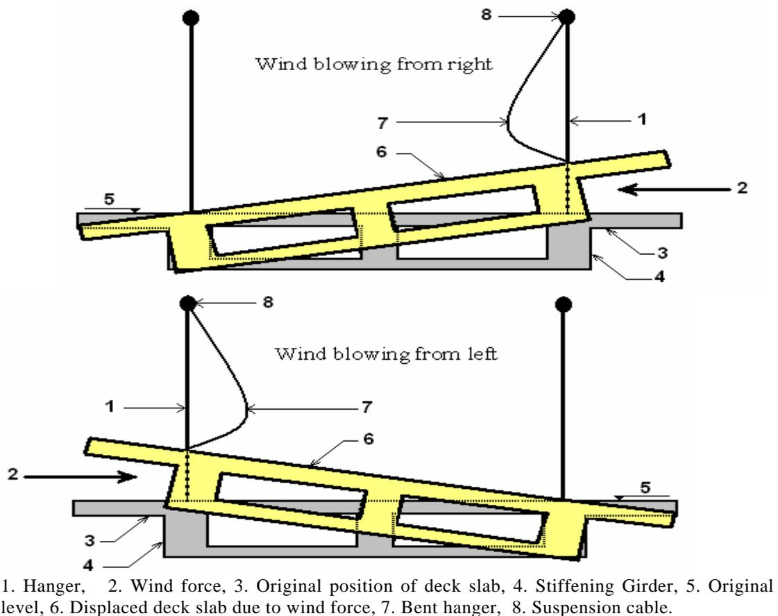
Fig. 1 Cross section showing the positions of a deck slab subjected to wind force.
