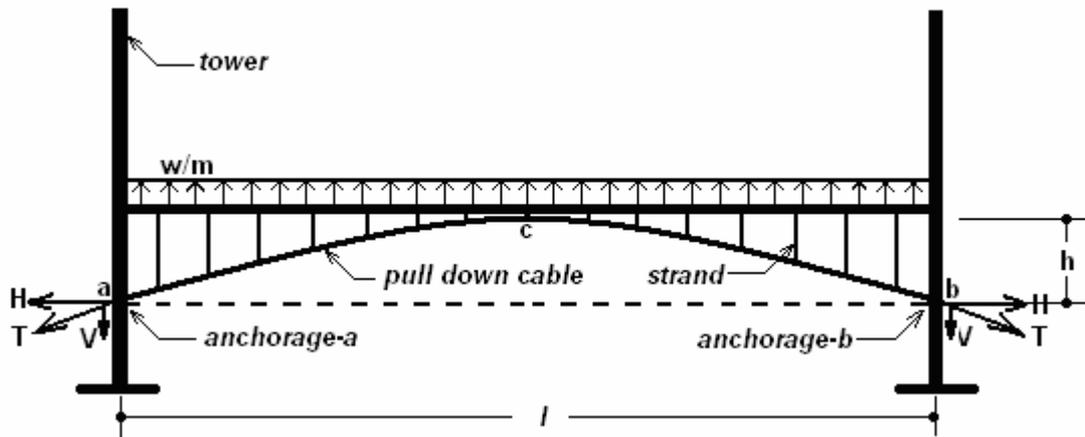
Fig. 4 Symbols, components and uniform loading of a Pull-down cable system.
