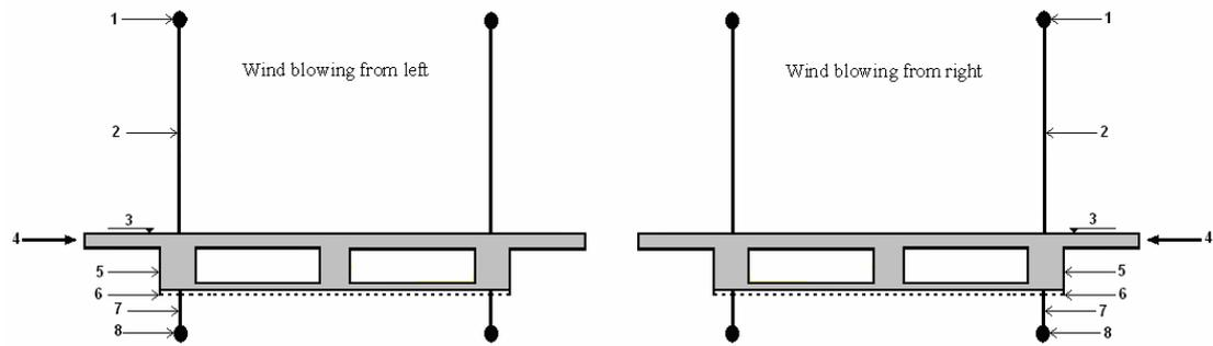
1. Suspension cable, 2. Hanger, 3. Original level, 4. Wind force, 5. Reduced Stiffening girder, 6. Original dimension, 7. Strand, 8. Pulling down cable.
