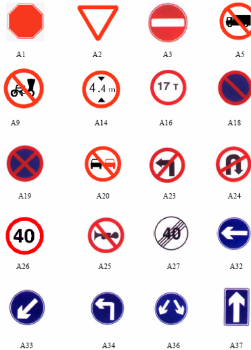
Figure 1. Twenty regulatory signs evaluated (shown with the sign designation by Roads and Highways Department, Govt. of Bangladesh).
