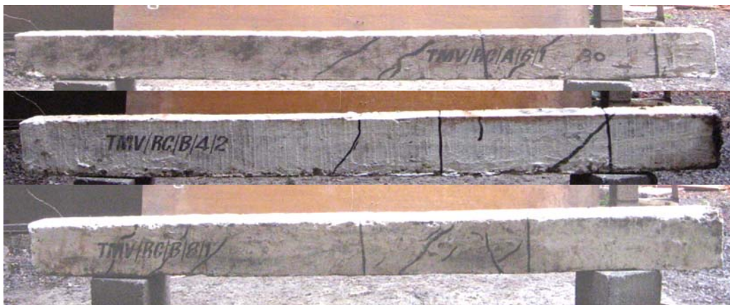
Figure 2. Typical failure patterns
