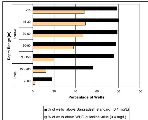
Figure 3. Distribution of manganese concentration water according to depth of w
