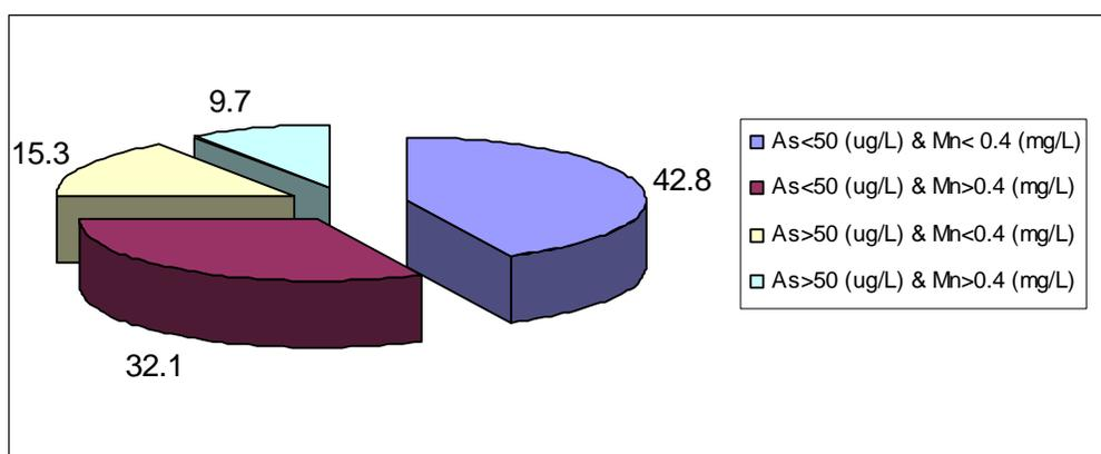
Figure 4. Status of wells with respect to arsenic and manganese concentrations
