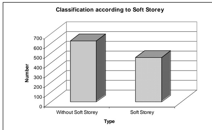
Figure 3b. Relation between numbers of buildings according to Soft Storey
