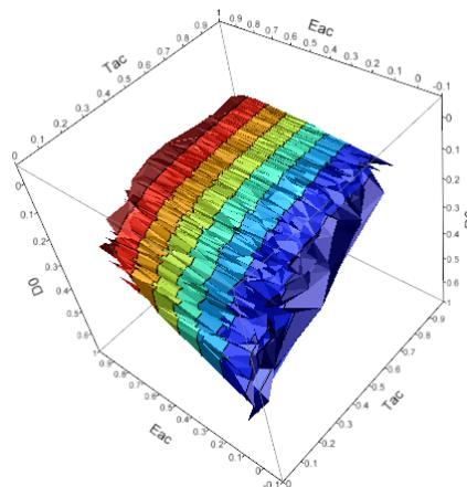
Figure 6. SVM predicted AC surface layer modulus ( $E_{AC}$ ) response surface as a function of AC surface layer thickness ( $T_{AC}$ ) and surface deflection at 0-mm radial offset from the center of the loading plate ( $D_0$ ).
