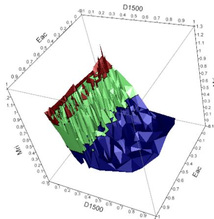
Figure 8. Subgrade layer elastic modulus ( $M_{Ri}$ ) as a function of AC surface layer elastic modulus ( $E_{AC}$ ) and surface deflection measured at 1500-mm radial offset from the center of the loading ( $D_{1500}$ ).
