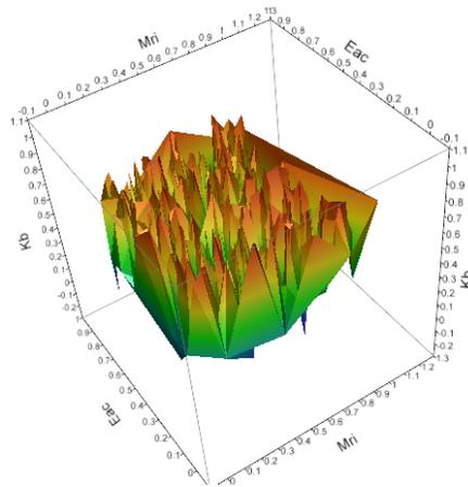
Figure 7. SVM predicted base layer modulus parameter ( $K_b$ ) response surface as a function of AC surface layer elastic modulus ( $E_{AC}$ ) and subgrade layer elastic modulus ( $M_{Ri}$ ).
