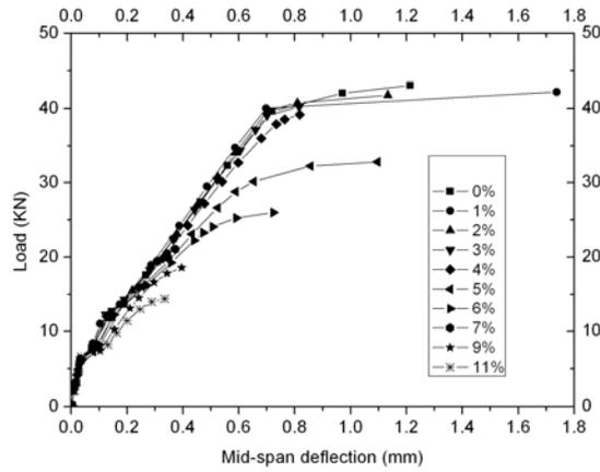
Figure 10. Load-displacement curves under different corrosion rates
