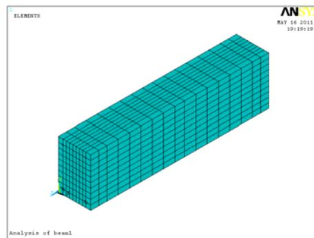
Figure 4. Concrete element model
