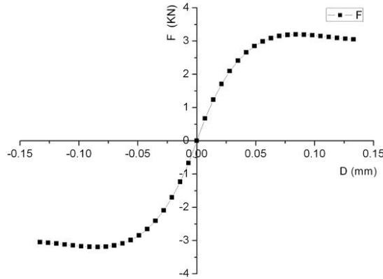
Figure1. The load-displacement relationship of the spring element along the longitudinal direction
