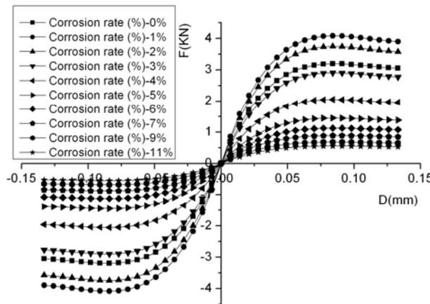
Figure 2.  $F$ - $D$  curves of the spring element along the longitudinal direction under the different corrosion rates
