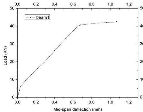
Figure 8. Load-deflection of the consolidated model
