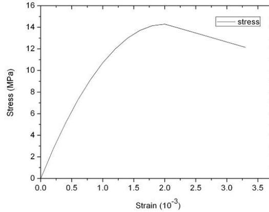
Figure 3. MISO curve of the concrete
