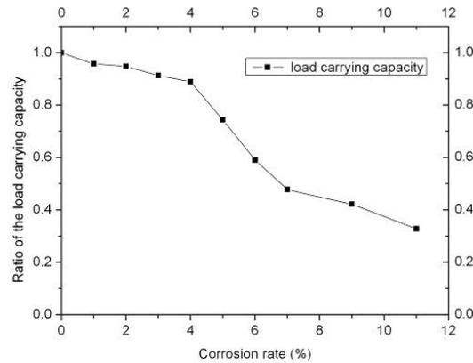
Figure 12. The effect of the corrosion on the load carrying capacity
