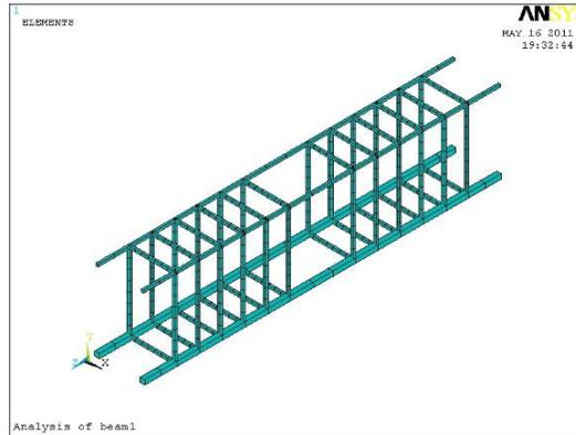
Figure 6. Bar element model
