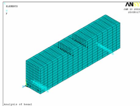
Figure 7. Consolidated supported beam model
