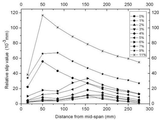
Figure 11. The effect of corrosion rate on the slip value at the bar-concrete interface
