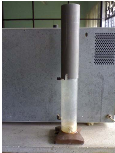
Figure 3. A typical setup for permeability test
