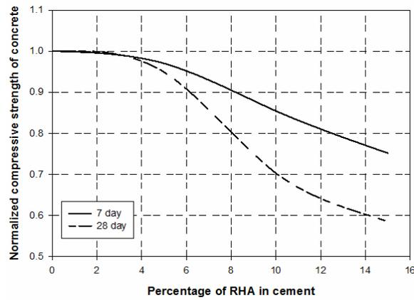
Figure 8. Effect of RHA on the compressive strength of concrete
