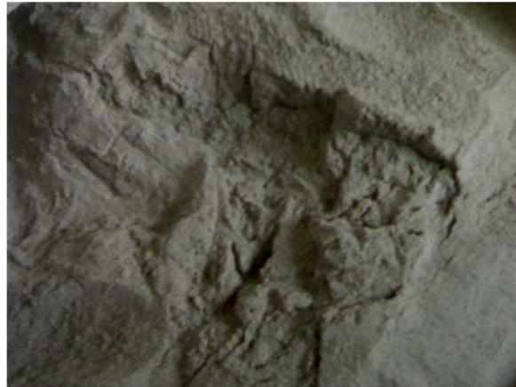
Figure 1. Rice husk ash after drying and sieving
