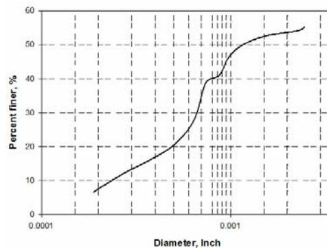
Figure 2. Grain size distribution of RHA used in this study
