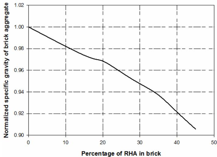
Figure 13. Effect of RHA on the specific gravity of brick aggregate
