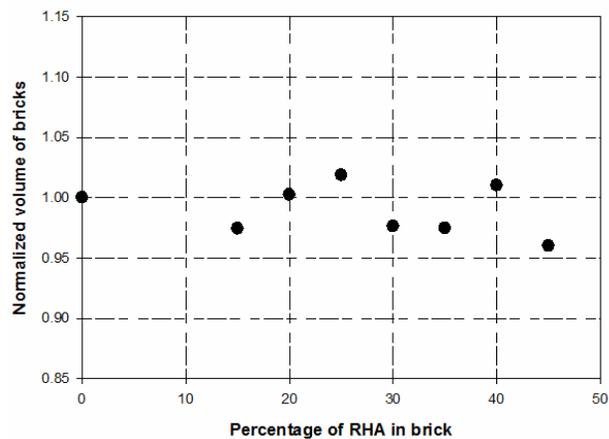
Figure 10. Effect of RHA on the volume of bricks.
