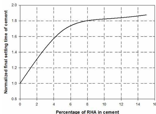
Figure 6. Effect of RHA on the final setting time of cement
