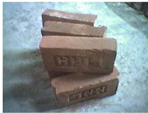
(b) Brick with partial replaced of clay with RHA
