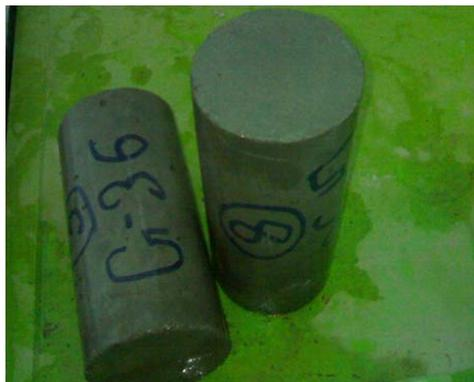
(a) Cylinder with partial replaced of cement with RHA
