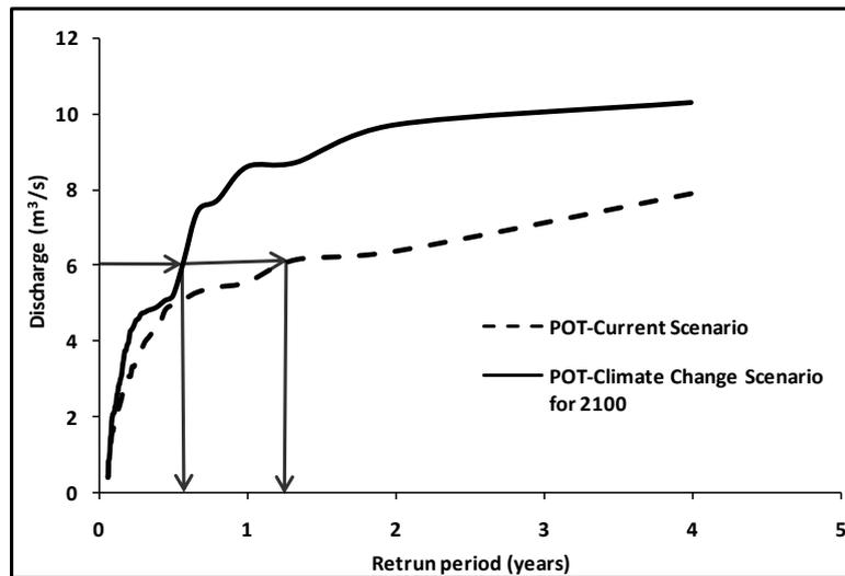
Fig. 7. Effect of climate change (high scenario) on peak runoff from two sub-catchments
