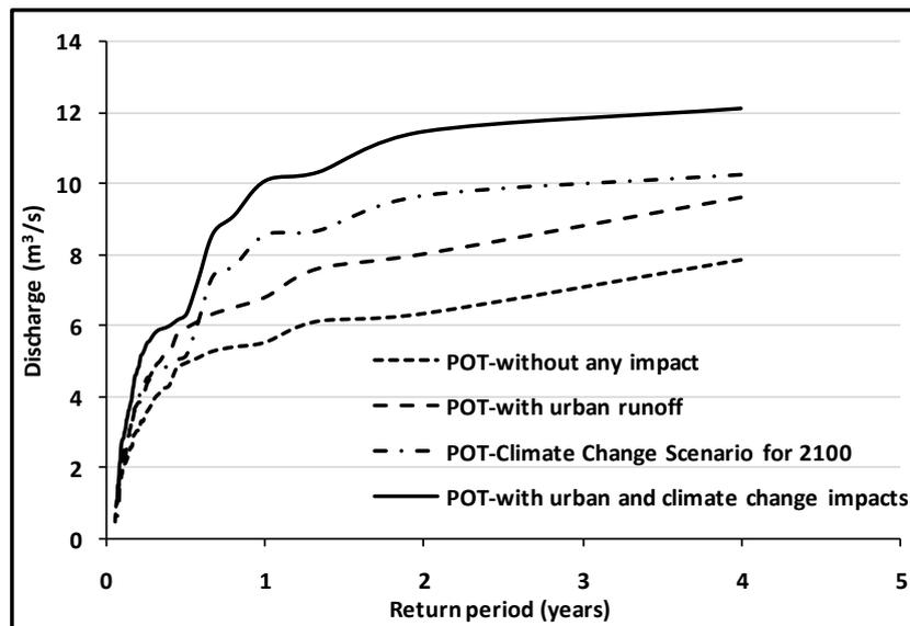
Fig. 9. Relative effect of urban runoff and climate change 'high' scenario both alone and together on peak runoff from two sub-catchments
