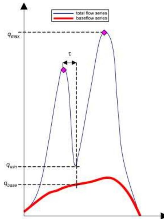
Fig. 3. Parameters for selecting nearly independent POT values (Adapted from Willems, 2009)
