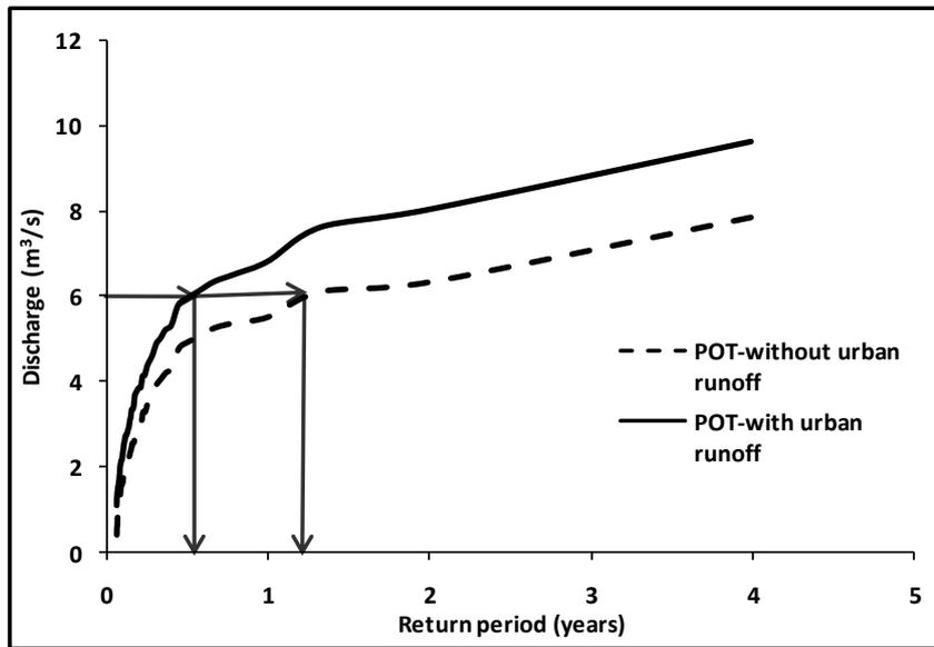
Fig. 6. Effect of urban runoff from the city on peak runoff from two sub-catchments
