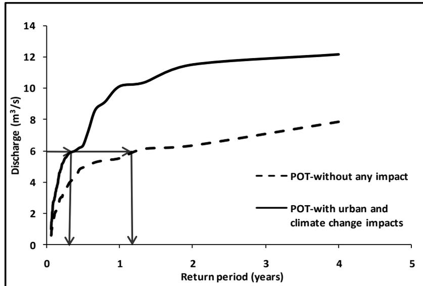
Fig. 8. Effect of both the urban runoff and climate change 'high' scenario on peak runoff from two sub-catchments
