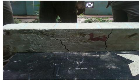
(b) Shear failure of RCC beam
