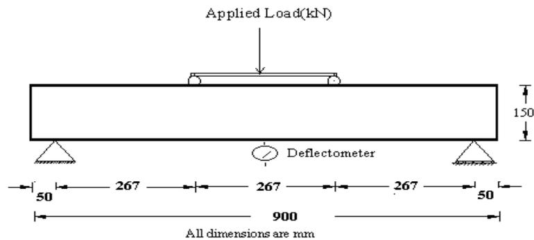
Fig. 1. Details of test beam
