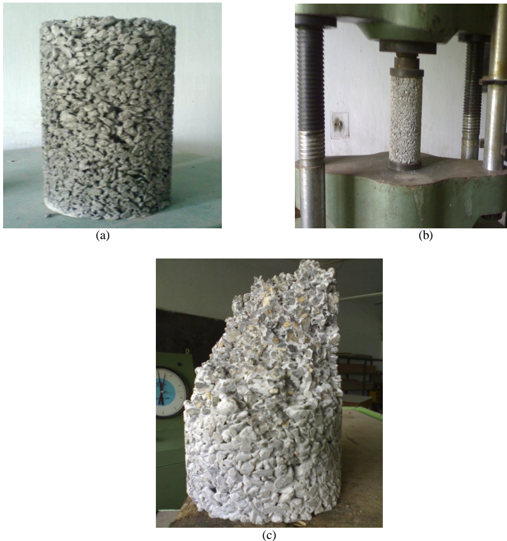
Fig 2. (a) A typical cylindrical specimen of pervious concrete (b) Specimen under loading (c) Failure pattern of specimen
