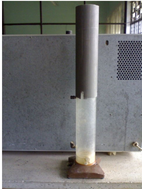
Fig 3. A typical setup for permeability test
