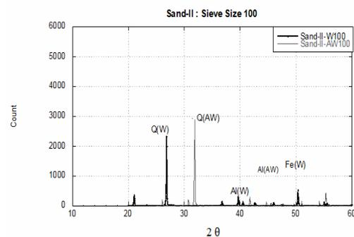
Fig. 22. X-ray diffraction of Sand II on grain size retained on #100
