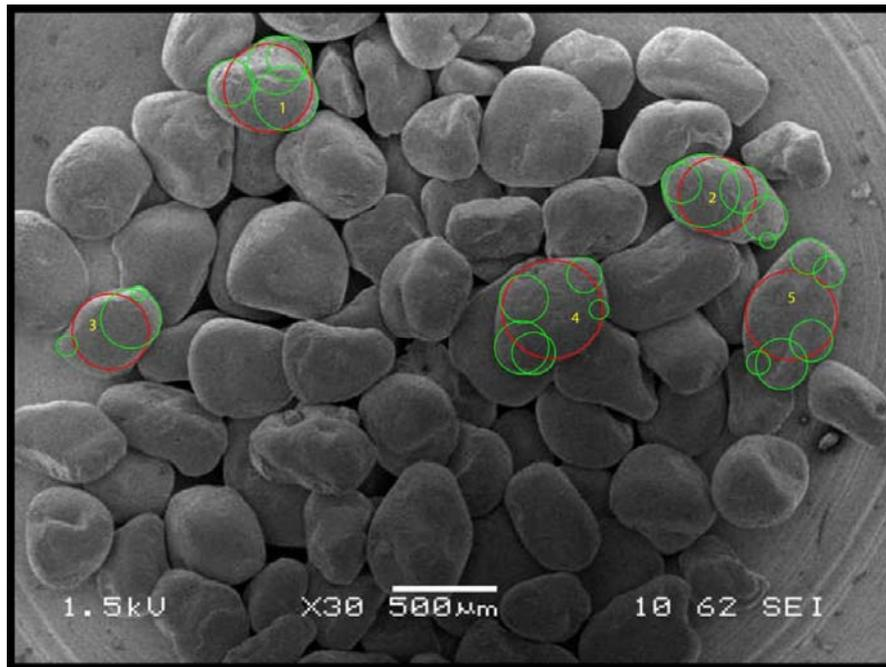
Fig. 23. Determination of roundness of Ottawa standard sand
