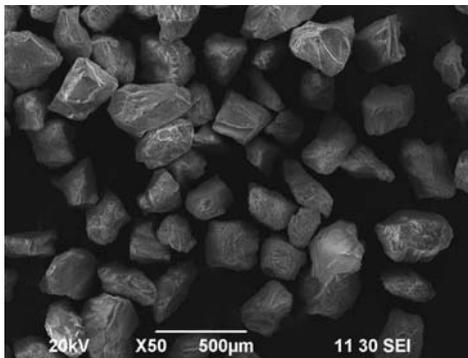
Fig. 15. Shape of Sand II W (#100)
