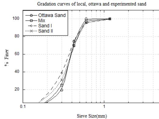
Fig. 8. Gradation curves of samples after processing
