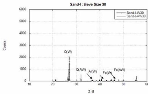
Fig. 17. X-ray diffraction of Sand I on grain size retained on #30
