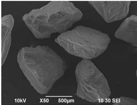
Fig. 13. Shape of Sand II W (#30)
