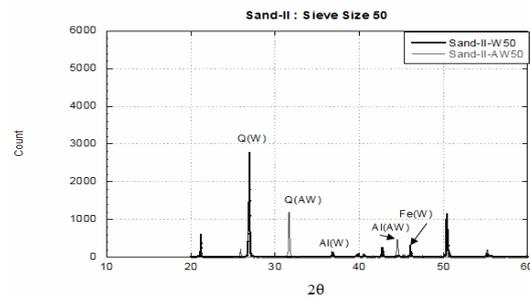
Fig. 20. X-ray diffraction of Sand II on grain size retained on #50
