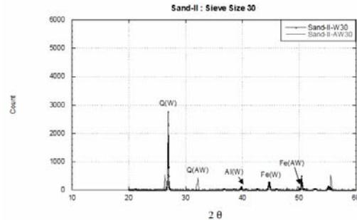
Fig. 18. X-ray diffraction of Sand II on grain size retained on #30
