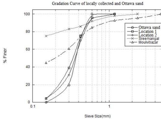
Fig. 7. Gradation curves of sand samples before processing
