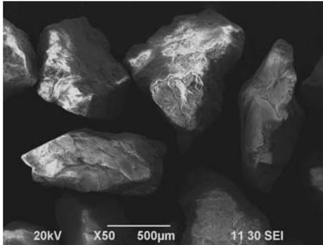
Fig. 9. Shape of Sand I W (#30)
