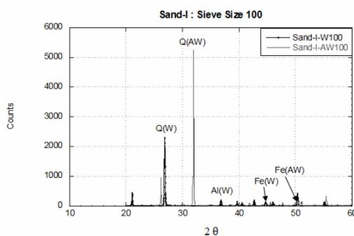
Fig. 21. X-ray diffraction of Sand I on grain size retained on #100
