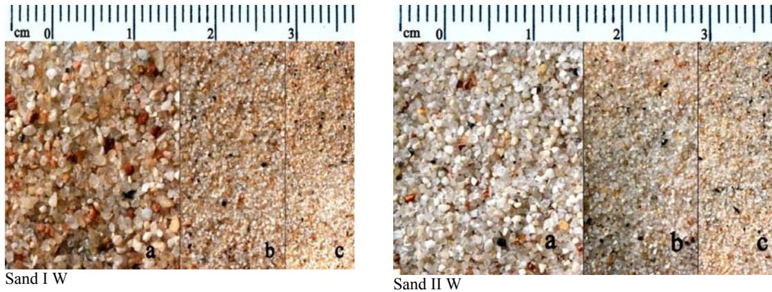
Fig. 6. Physical appearance of Sands at different grain sizes (a) Material retained on Sieve #30, (b) Material retained on Sieve #50, (c) Material retained on Sieve #100
