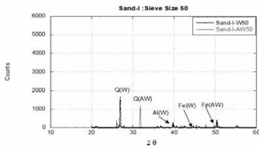
Fig. 19. X-ray diffraction of Sand I on grain size retained on #50
