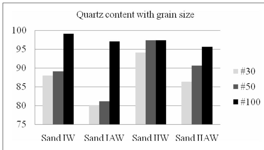
Fig. 25. Variation of quartz content with grain size in different sand
