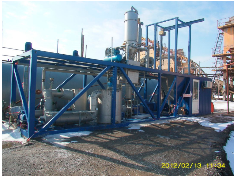
Fig.7. Photograph of a Sasobit mixing plant in Baku, Azerbaijan
