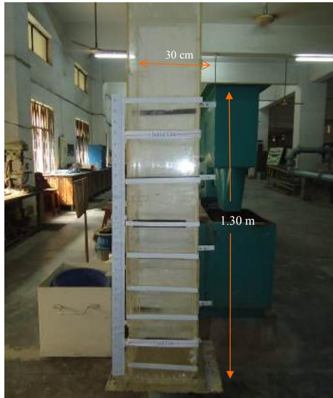
Photograph 1: Plexiglas settling column in the Hydraulics and River Engineering Laboratory, BUET
