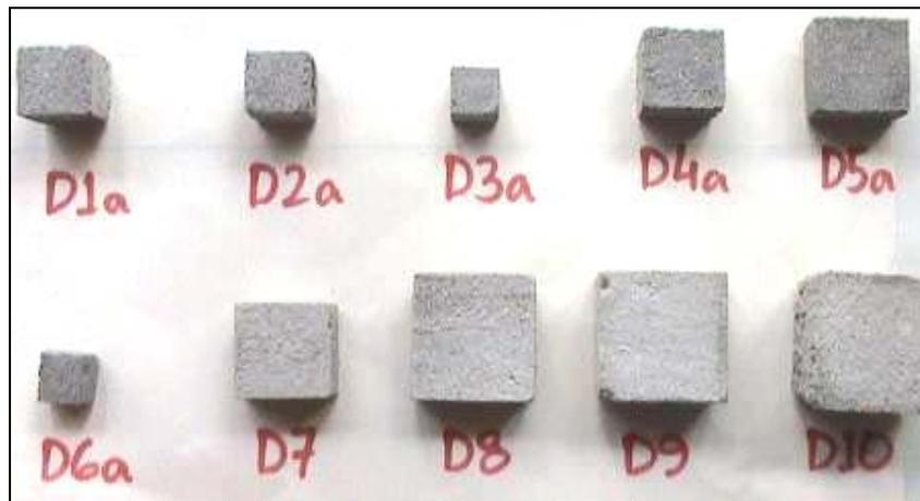
Photograph 2: Various sizes of sand cement block used in the study
