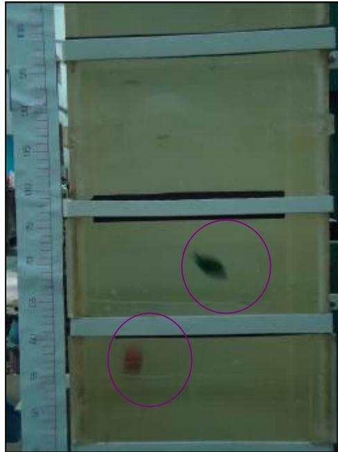
Photograph 4: Sand cement block is falling faster than geobag in the settling column
