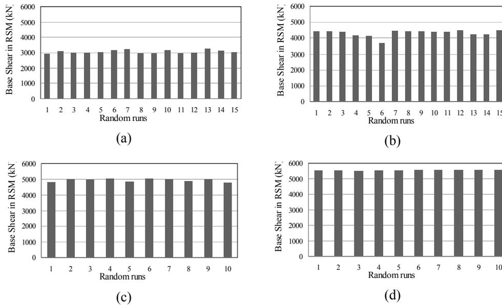
Fig. 4 Variation in base shear value (RSM) of 12 storied building (EQ load in X-dir) for random infill pattern with no infill on Ground floor and (a) 20%, (b) 40%, (c) 60%, (d) 80% infill on upper floors.
