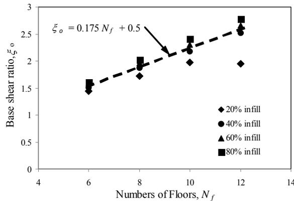
Fig. 8 Base shear ratio,  $\beta_o$ , as a function of number of floors and percent amount of infill
