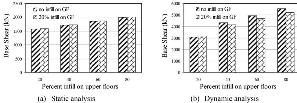
Fig. 6. Comparison of base shear for no infill and 20% infill at ground floor level.
