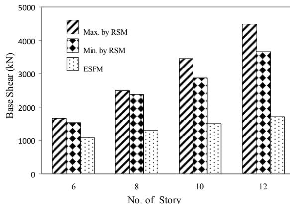
Fig. 5 Comparison of static and dynamic base shear for 40% infill on upper floors and no infill on ground floor.
