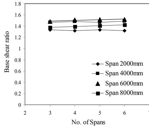
Fig. 7. Base shear ratio for different number of spans for a 6 storied building with 40% infill on upper stories and no infill on GF
