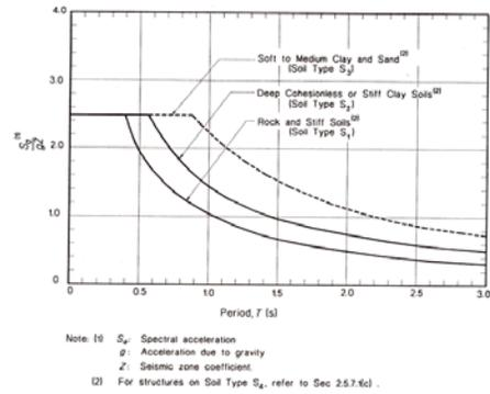
Fig.2.2 Normalized response spectra for 5% damping ratio.
