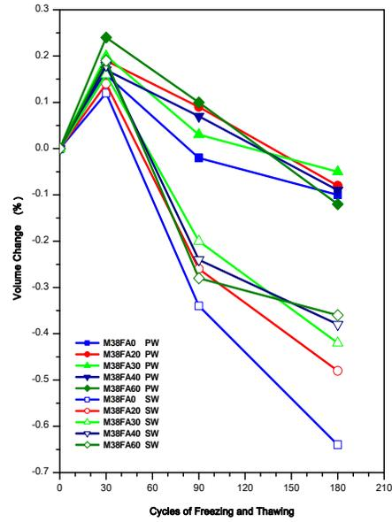
Fig.4: Volume Change - Freeze Thaw Relation for M38 Grade Concrete
