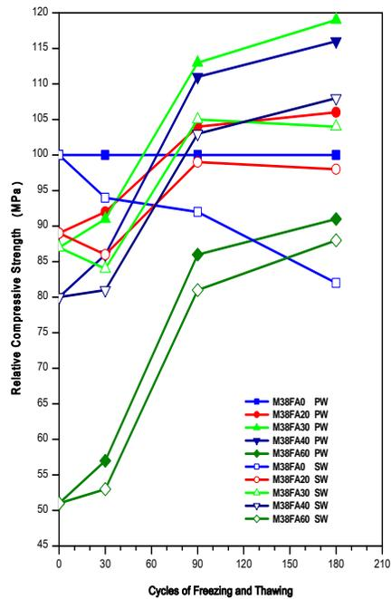
Fig.10: Relative Compressive Strength - Freeze Thaw Relation for M38 Grade Concrete
