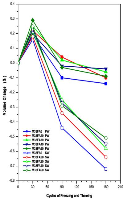
Fig.5: Volume Change - Freeze Thaw Relation for M33 Grade Concrete
