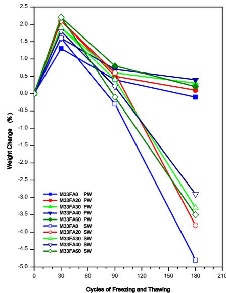
Fig.2: Weight Change - Freeze Thaw Relation for M33 Grade Concrete
