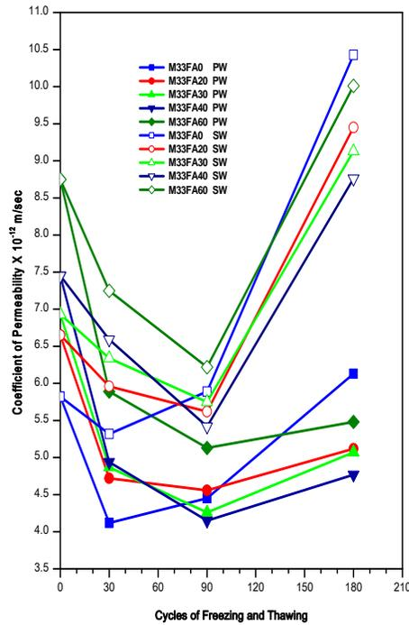
Fig.14: Permeability - Freeze Thaw Relation for M33 Grade Concrete
