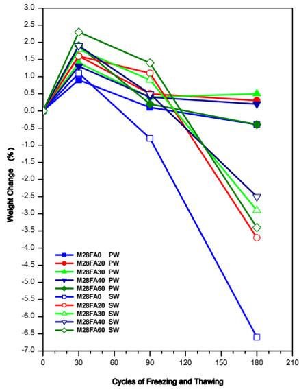
Fig.3: Weight Change - Freeze Thaw Relation for M28 Grade Concrete
