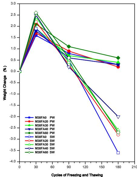
Fig.1: Weight Change - Freeze Thaw Relation for M38 Grade Concrete
