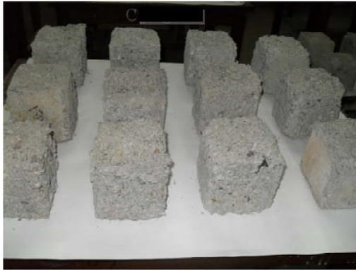
Plate no. 4: Concrete specimens after 90 cycles of freezing and thawing in PW
