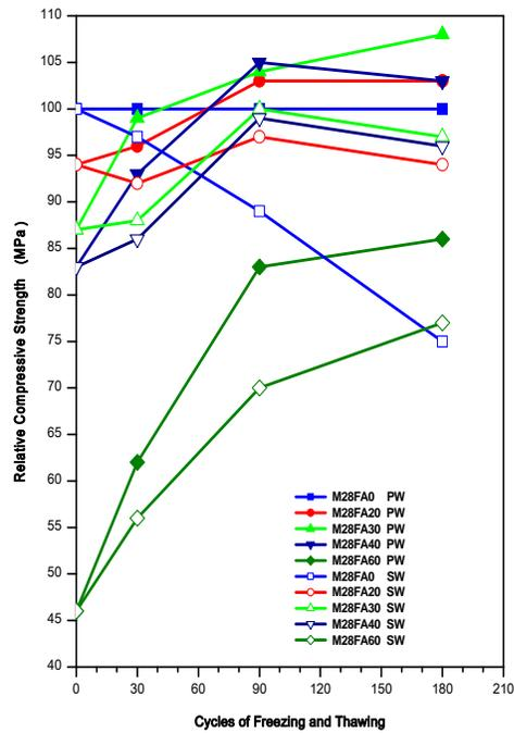
Fig.12: Relative Compressive Strength - Freeze Thaw Relation for M28 Grade Concrete
