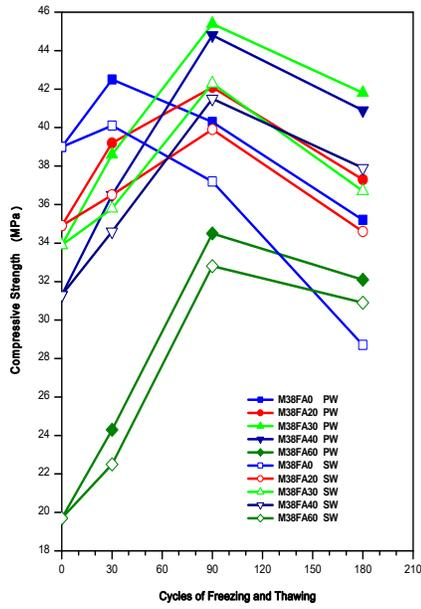
Fig.7: Compressive Strength - Freeze Thaw Relation for M38 Grade Concrete
