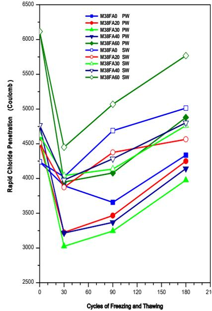
Fig.16: Rapid Chloride Penetration - Freeze Thaw Relation for M38 Grade Concrete
