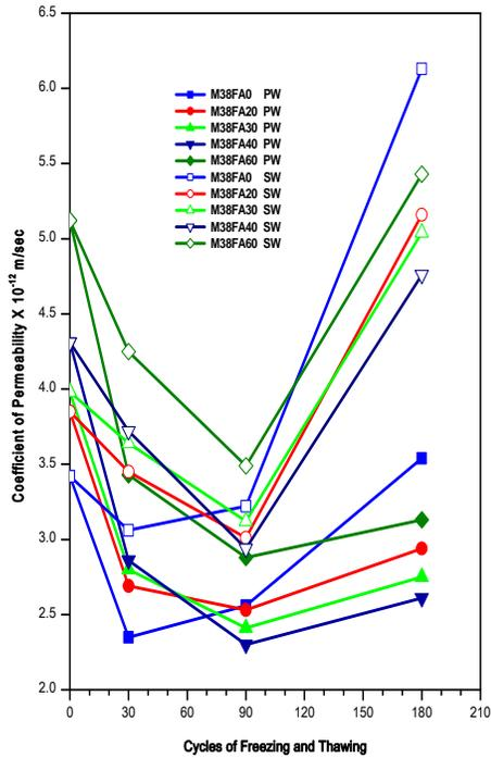
Fig.13: Permeability - Freeze Thaw Relation for M38 Grade Concrete
