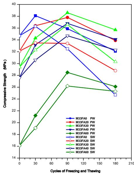
Fig.8: Compressive Strength - Freeze Thaw Relation for M33 Grade Concrete
