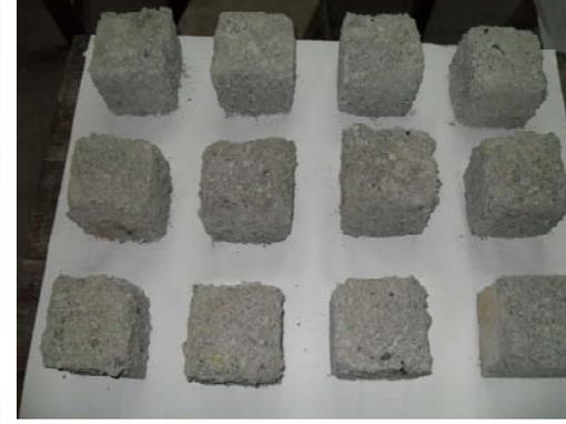
Plate no. 5: Concrete specimens after 90 cycles of freezing and thawing in SW
