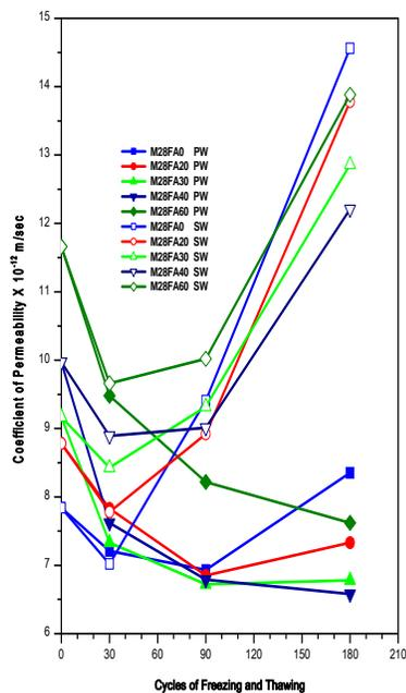
Fig.15: Permeability - Freeze Thaw Relation for M28 Grade Concrete
