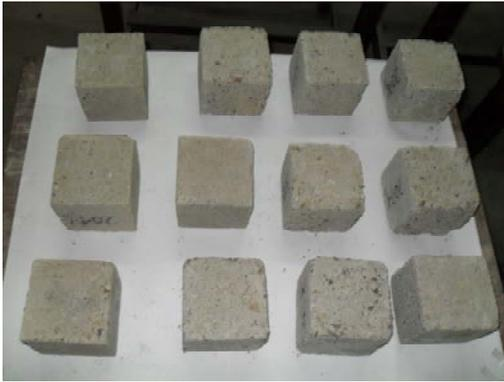
Plate no. 2: Concrete specimens after 30 cycles of freezing and thawing in PW
