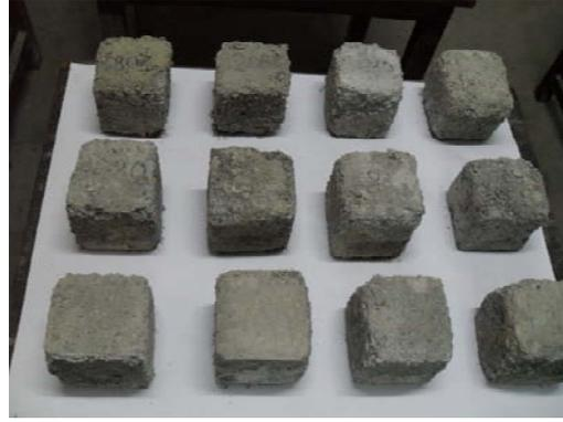
Plate no. 3: Concrete specimens after 30 cycles of freezing and thawing in SW
