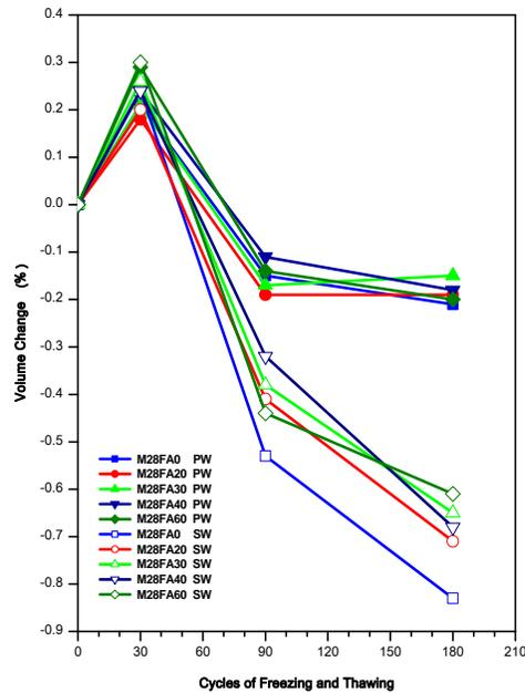
Fig.6: Volume Change - Freeze Thaw Relation for M28 Grade Concrete
