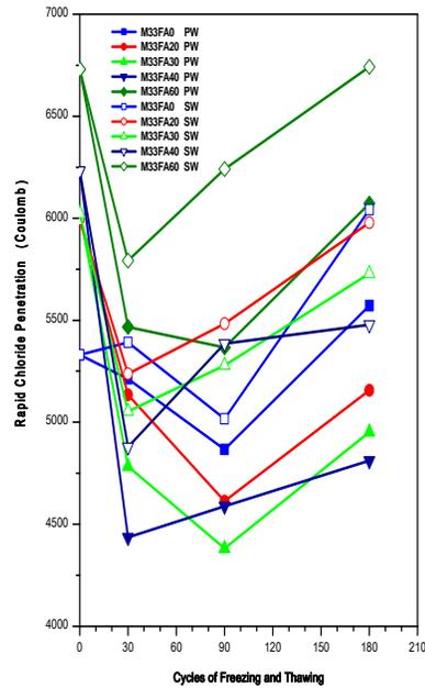
Fig.17: Rapid Chloride Penetration - Freeze Thaw Relation for M33 Grade Concrete
