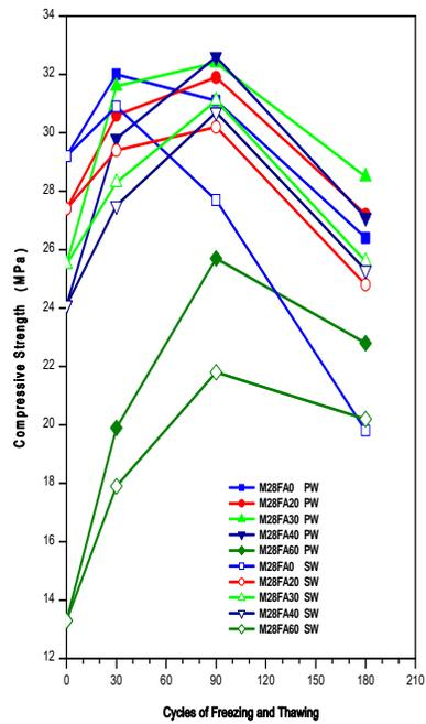
Fig.9: Compressive Strength - Freeze Thaw Relation for M28 Grade Concrete
