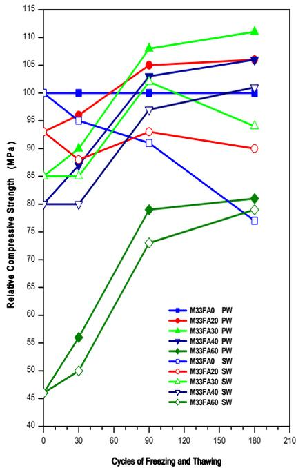
Fig.11: Relative Compressive Strength - Freeze Thaw Relation for M33 Grade Concrete
