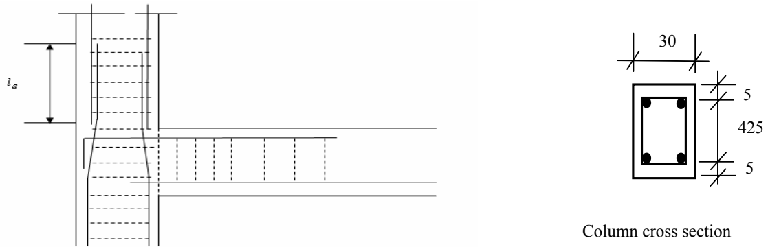
Fig.3. Beam column joint
