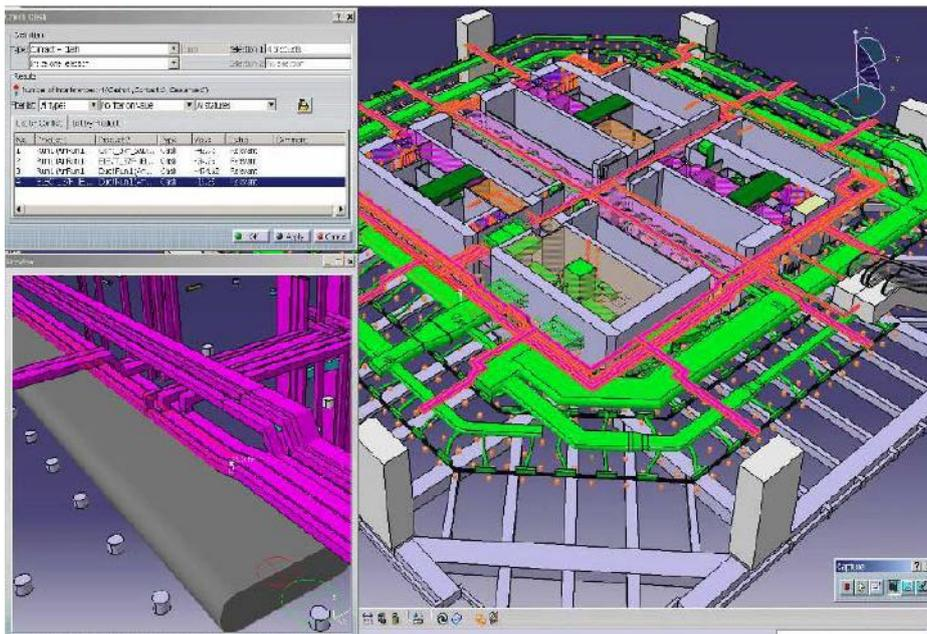
Fig. 9. Automated Clash Detections in OIE Project (Gammon Construction Ltd, HK)
