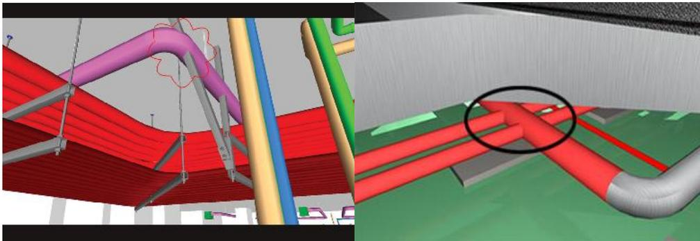
Fig. 7. Clash Detection by BIM software
