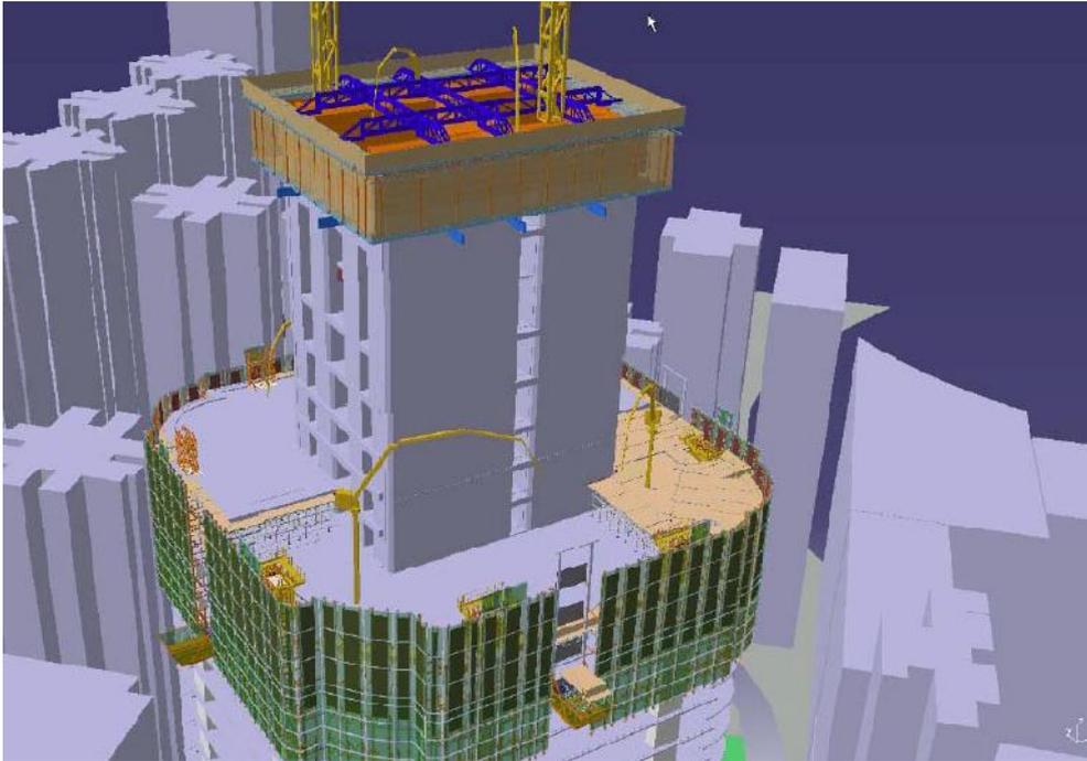
Fig. 12. Construction Sequencing Model (Gammon Construction Ltd, HK)
