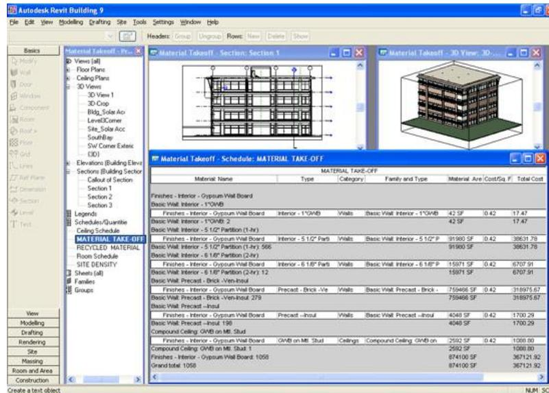
Fig. 7. Automatic Cost Estimation by BIM software
