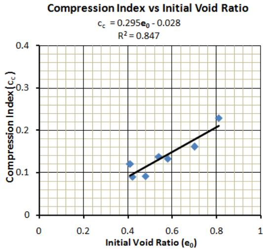
Fig. 27. Correlation between Compression Index & Initial Void Ratio at Bhulta, Narayanganj.
