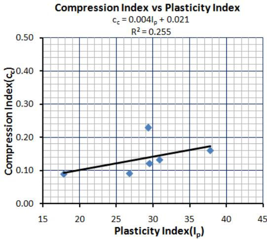
Fig. 25. Correlation between Compression Index & Plasticity Index at Bhulta, Narayanganj.
