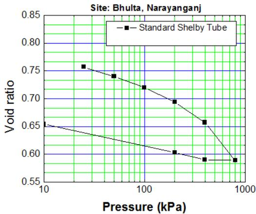
Fig. 15. Typical e-log p curve of samples collected from Bhulta, Narayanganj.
