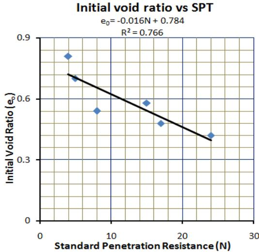
Fig. 19. Relationship between Initial Void ratio & SPT at Bhulta, Narayanganj.
