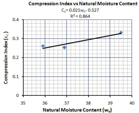
Fig. 30. Correlation between Compression Index & Natural Moisture Content at AMC, Khulna.
