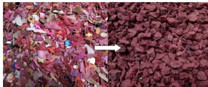
Fig. 1. Shredded raw plastic materials to Recycled plastic aggregate.
