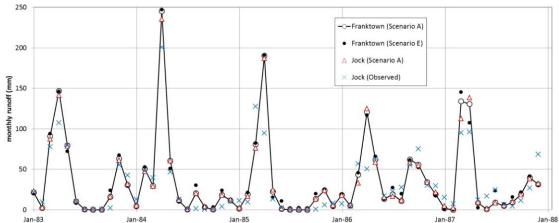
Fig. 10. Variation of monthly runoff for Franktown basin and Jock watershed at Moodie Drive; the effect of wetland removal is evident between Scenarios A and E; the Jock values provide and benchmark for comparison and also give an indication of the accuracy of simulated values.
