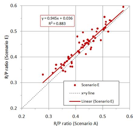
Fig. 9. Annual runoff to precipitation ratio for Franktown basin under existing condition (Scenario A) and when all wetlands are removed (Scenario E).
