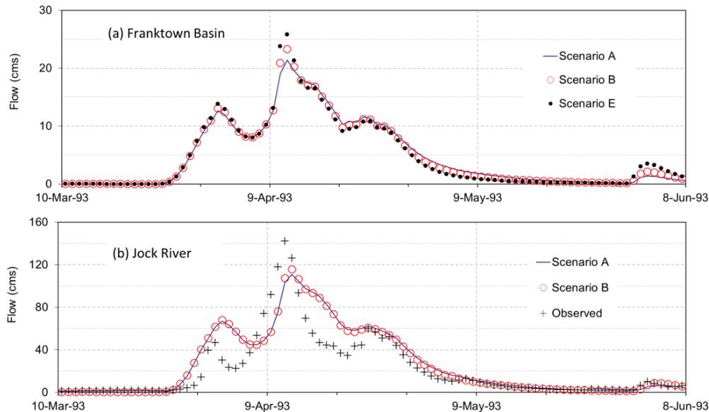
Fig. 5. Typical spring-time hydrographs at (a) Franktown basin and (b) Jock River near its outlet at Moodie Drive; Scenarios A, B and E illustrate the effect of wetland removal; the measured values indicate the ability of Mike11 model to simulate Jock basin hydrology.
