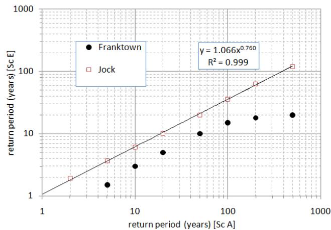
Fig. 19. Recurrence reduction at Franktown basin and Jock watershed; the return period of a flood quantile under existing condition (Scenario A, plotted along the x axis) reduced considerably when wetlands are removed (Scenario E, plotted along y axis); for instance, the existing 1:100 year flood for Franktown basin becomes only a 1:15 year flood.
