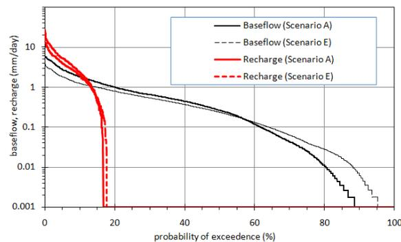
Fig. 16. Flow duration curves for base flow and groundwater recharge; comparison of Scenarios A and E reveals the effect of wetland removal.
