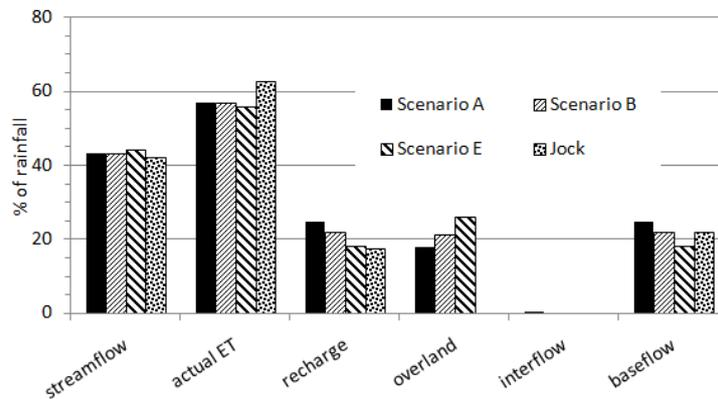
Fig. 8. Overall annual water budget components of Franktown basin as computed from 59 years of model output (1945-2003); the Jock basin values were computed for 1974-2003 by MRSR (2011) and provide a yardstick for comparison; note that simulated interflow is very small and was not available for Jock.
