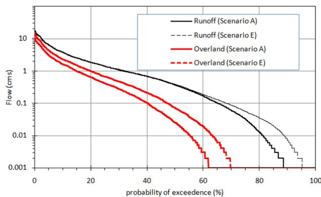
Fig. 13. Flow duration curves for total runoff and overland flow; comparison of Scenarios A and E reveal the effect of wetland removal.
