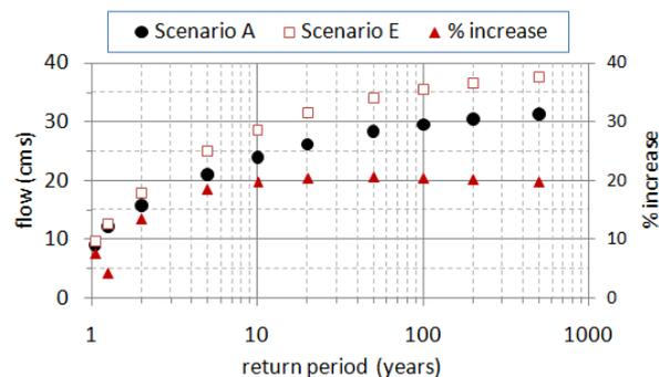
Fig. 17. Frequency analysis of total runoff or stream flow generated by Franktown basin; wetland removal is expected to increase the 1:100 flood by 20%.
