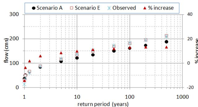
Fig. 18. Frequency analysis of stream flow of the Jock River at Moodie Drive; wetland removal is expected to increase the 1:100 flood by 12%; flood quantiles based the simulated values under existing conditions (Scenario A) are about 10% lower than those based on observation.
