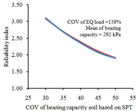
Fig. 4. Effect of COV of soil on the reliability of footings under earthquake loads using F.S=2.50
