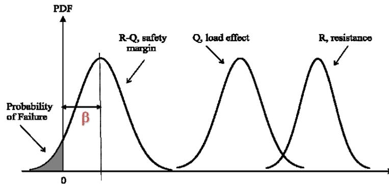
Fig. 2. Failure probability, load effect and resistance effect.
