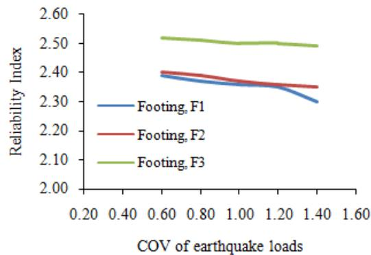
Fig. 9. Effect of COV of earthquake load on the reliability of footings using COV of soil capacity of 40% for Model building-2 using a F.S = 2.50
