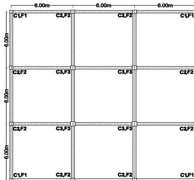
Fig. 1. Beam column grid of model building.
