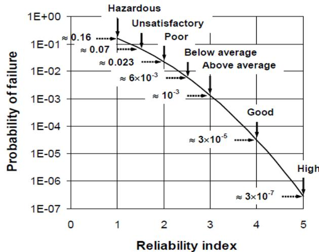
Fig. 3. Relationship between reliability index  $\beta$  and probability of failure  $p_f$
