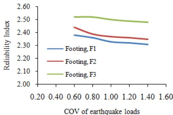
Fig. 8. Effect of COV of earthquake load on the reliability of footings using COV of soil capacity of 40% for Model building-1 using a F.S = 2.50
