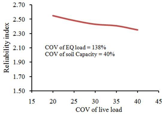
Fig. 6. Effect of COV of live load on the reliability of footings under earthquake load using F.S = 2.50
