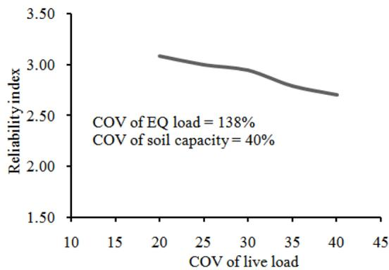
Fig. 7. Effect of COV of live load on the reliability of footings against punching shear failure under earthquake loads using a F.S=2.50
