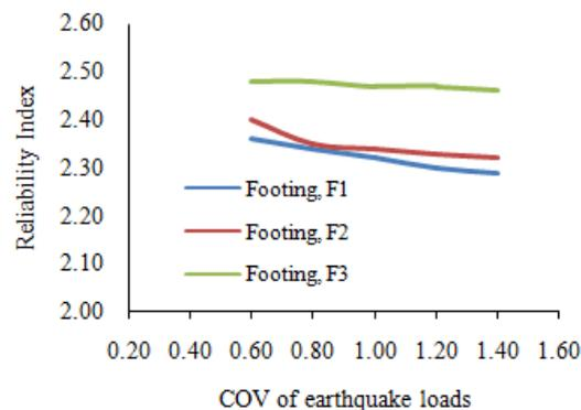
Fig. 10. Effect of COV of earthquake load on the reliability of footings using COV of soil capacity of 40% for Model building-3 using a F.S = 2.50
