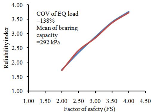
Fig. 5. Effect of factor of safety on the reliability of footings under earthquake load.
