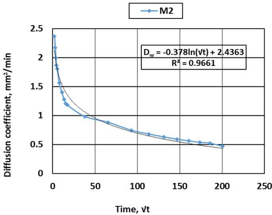
Water diffusion coefficient in cubes for Mix type (M2)
