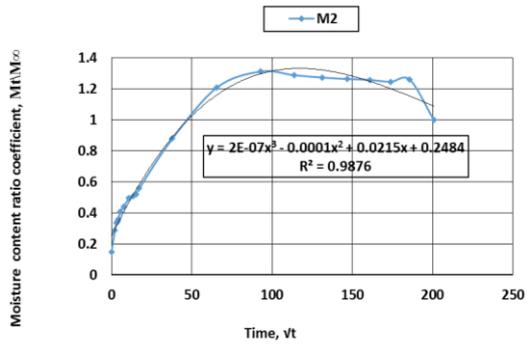
Moisture content ratio coefficient variation in cubes for Mix type (M2)
