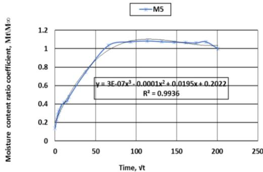
Moisture content ratio coefficient variation in cubes for Mix type (M5)
