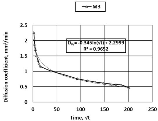
Water diffusion coefficient in cubes for Mix type (M3)
