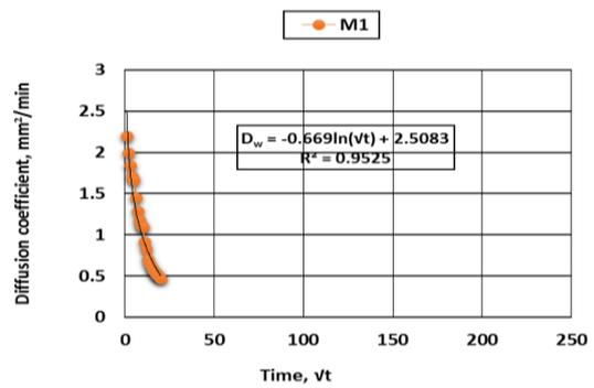
Water diffusion coefficient in cubes for Mix type (M1)
