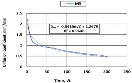
Water diffusion coefficient in cubes for Mix type (M5)
