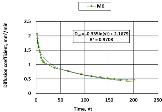
Water diffusion coefficient in cubes for Mix type (M6)
