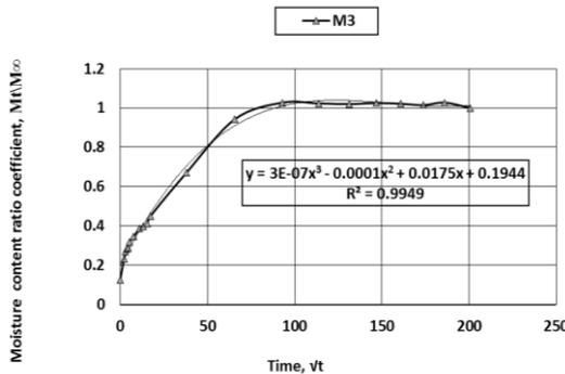
Moisture content ratio coefficient variation in cubes for Mix type (M3)
