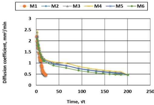
Water diffusion coefficient in cubes for different Mix types
