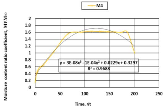
Moisture content ratio coefficient variation in cubes for Mix type (M4)
