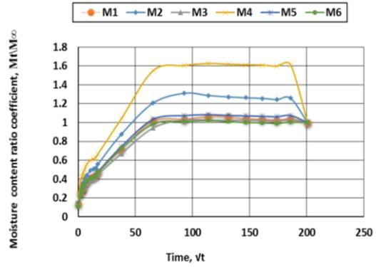
Moisture content ratio coefficient variation in cubes for Mix types
