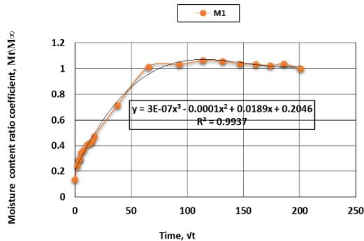
Moisture content ratio coefficient variation in cubes for Mix type (M1)
