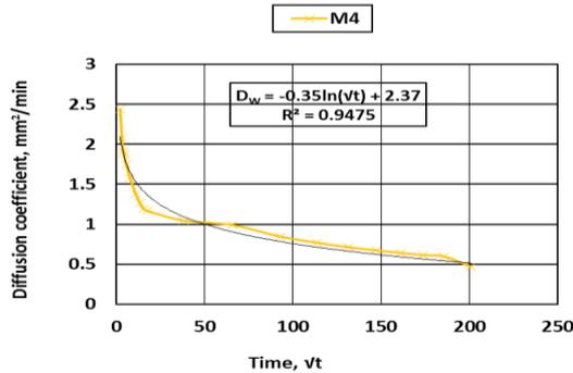
Water diffusion coefficient in cubes for Mix type (M4)
