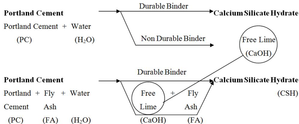
Fig. 1. Hydration mechanism of fly ash concrete.
