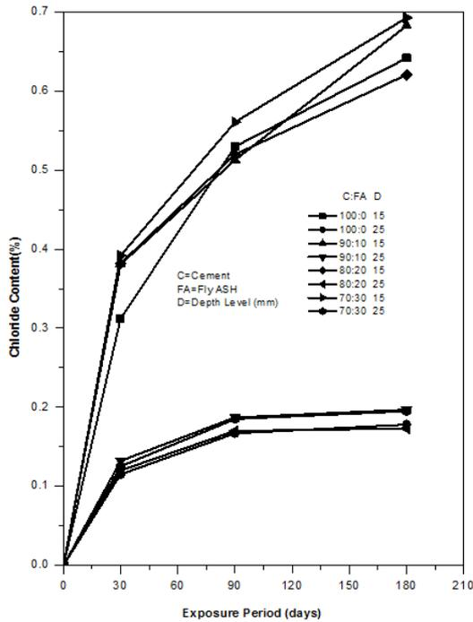
Fig. 8. Chloride content-exposure time relation for fly ash concretes exposed to sea water of 10T concentration.
