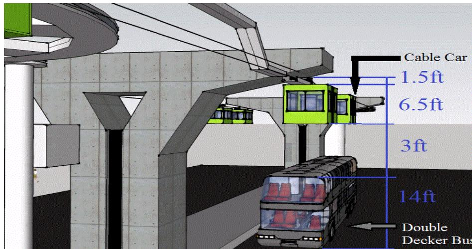
Fig. 6. Available height from the installation level up to the existing ground level.
