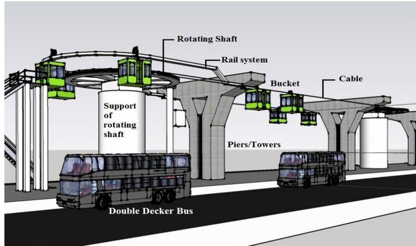
Fig. 7. Overall components of the proposed ropeway with base stations.
