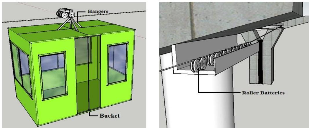
Fig. 8. The vehicle, hanger & roller batteries of the proposed ropeway.
