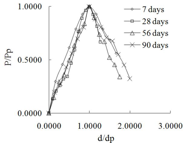
Fig. 4. Normalized stress-strain curve for the reference mix FA30RM70MD08 at different curing.
