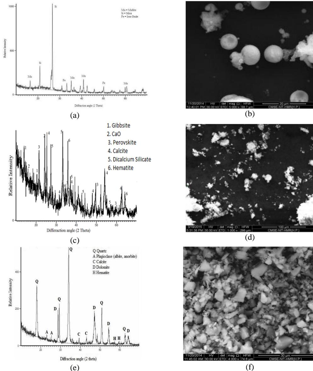
Fig. 1. (a) X.R.D of flyash, (b) SEM of fly ash (30kV, X5000, 20 $\mu$ m), (c) X.R.D of redmud (d) SEM of redmud (30KV, X1000, 100 $\mu$ m), (e) X.R.D of marble dust, (f) SEM of marble dust(30kV, X4000, 74.6 $\mu$ m).
