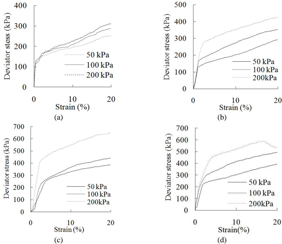
Fig. 6. Variation of deviator stress-axial strain for the reference mix at different confining pressures and at curing period of (a) 7 days (b) 28 days (c) 56 days and (d) 90 days.
