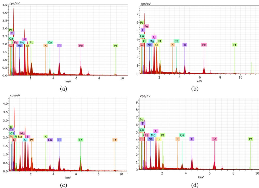
Fig. 9. Energy dispersive X-ray spectroscopy results on reference mix after (a) 7 days (b) 28 days (c) 56 days (d) 90 days of curing.
