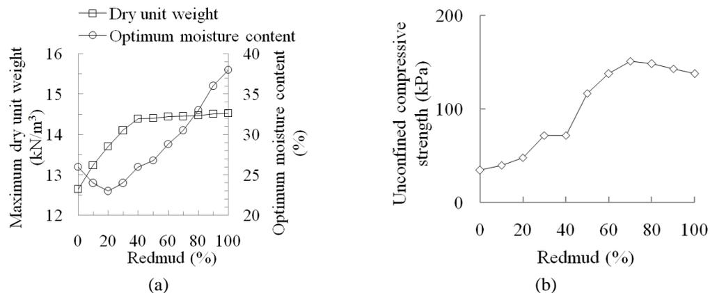
Fig. 2. (a) Variation of moisture content and maximum dry unit weight with varying percentage of redmud (b) Variation of unconfined compressive strength with percentage of redmud.
