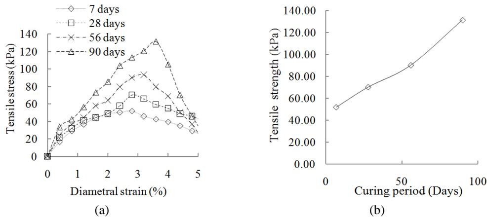
Fig. 8. (a) Tensile stress-diametral strain curves for the reference mix at different curing period (b) Variation of tensile strength for the reference mix with curing period.
