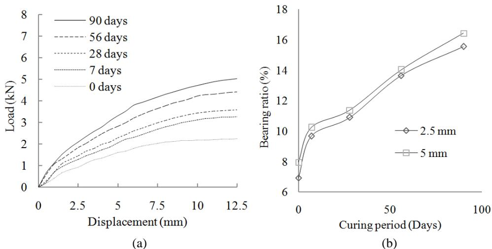
Fig. 5. (a) Load-displacement curves for the reference mix with curing period, (b) Variation of bearing ratio for the reference mix with curing period.
