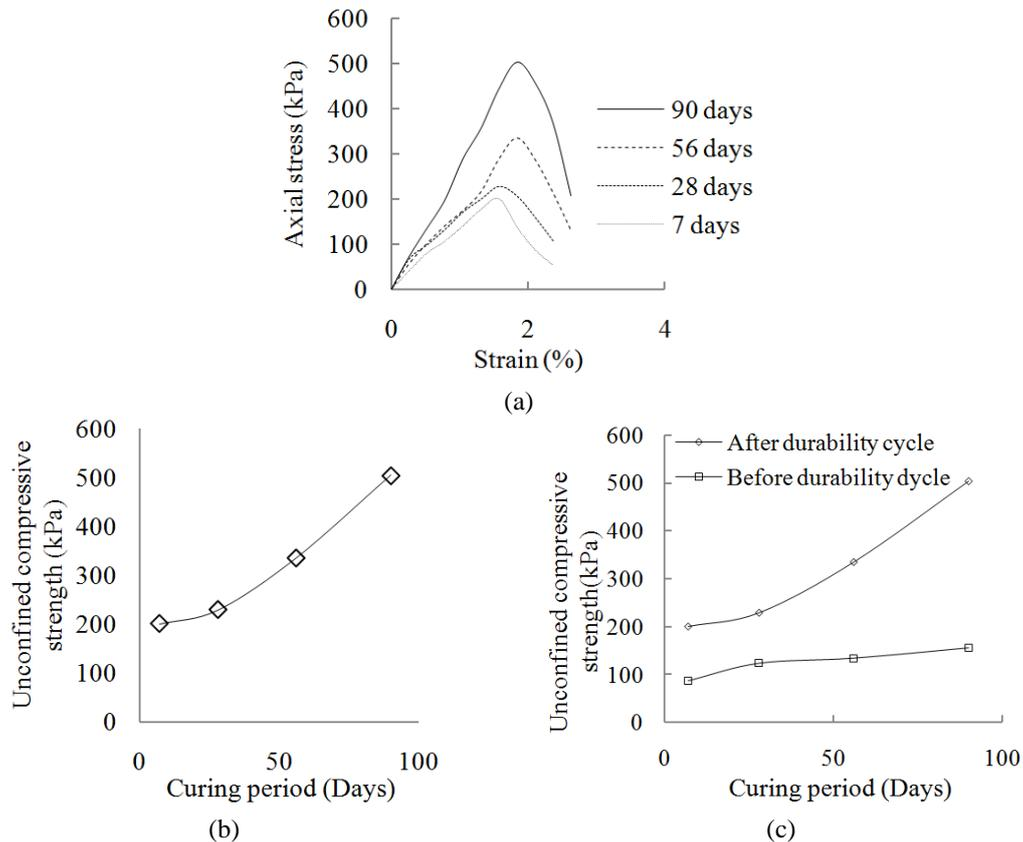
Fig. 7. (a) Axial stress-strain curves for the reference mix at different curing periods after the durability cycles (b) Variation of unconfined compressive strength after the durability cycles of the reference mix with curing period (c) Comparison of the unconfined compressive strength before and after the durability cycles.
