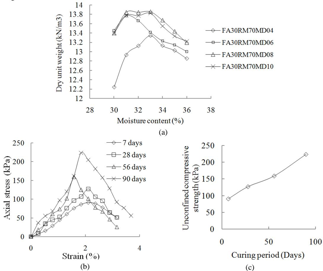
Fig. 3. (a) Compaction curves for the mix FA30RM70MD08 (b) Axial stress- strain curve for the mix FA30RM70MD08with curing period (c)Variation of unconfined compressive strength for the reference mix with curing period.
