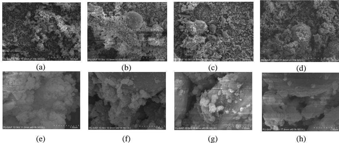
Fig. 10. Field emission scanned electron micrograph of the reference mix at (a) 7 days (10 kV 11mm×1.00k 50 um) (b) 28 days (10 kV 10.9mm×1.00k 50 um) (c) 56 days (10 kV 18.4mm×1.00k 50 um) (d) 90 days (10 kV 17.8mm×1.00k 50 um) (e) 7 days (10 kV 11mm×40.00k 1.0 um) (f) 28 days (10 kV 10.9mm×40.00k 1.0 um) (g) 56 days (10 kV 18.4mm×40.00k 1.0 um) (h) 90 days (10 kV 17.8mm×40.00k 1.0 um)
