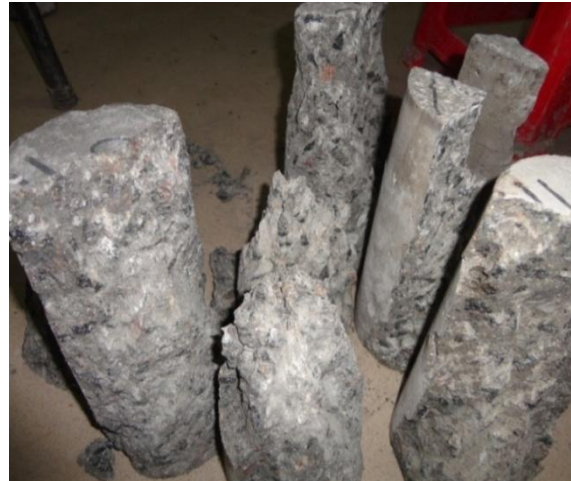
Fig. 14. Fracture surfaces of specimens.
