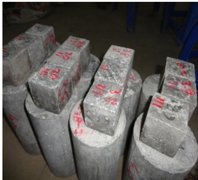
Fig. 1. Partial view of the cylinder and cube specimens.
