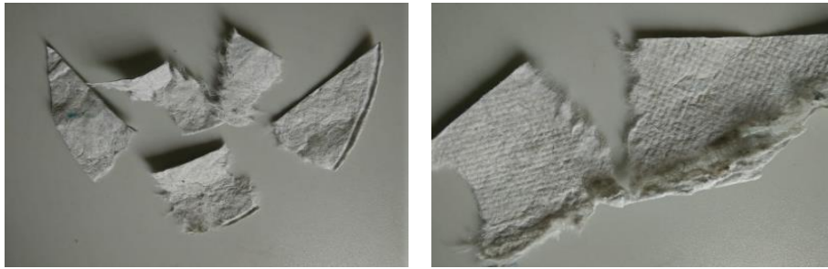
Fig. 4.7. Fibrous formation in torn paper pieces.
