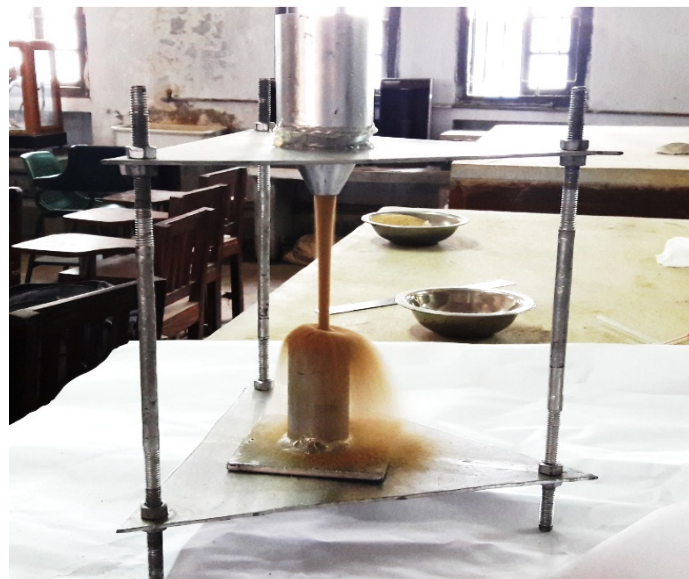
Fig. 7. Fine aggregate angularity (FAA) test in progress.
