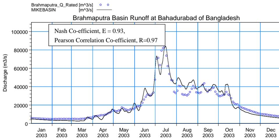
Fig. 2. Comparison of model runoff with rated discharge at Bahadurabad for 2003.
