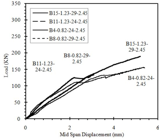
Fig. 4(b). Load-Displacement Curves of RC Beams – Shear-Span-to-Depth Ratio = 2.45
