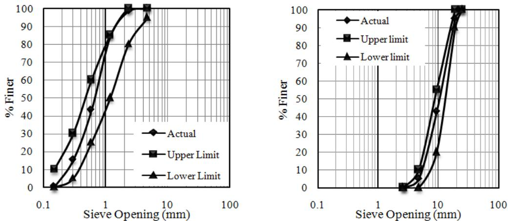
Fig. 1. Grading curves of fine aggregate and coarse aggregate (BA).
