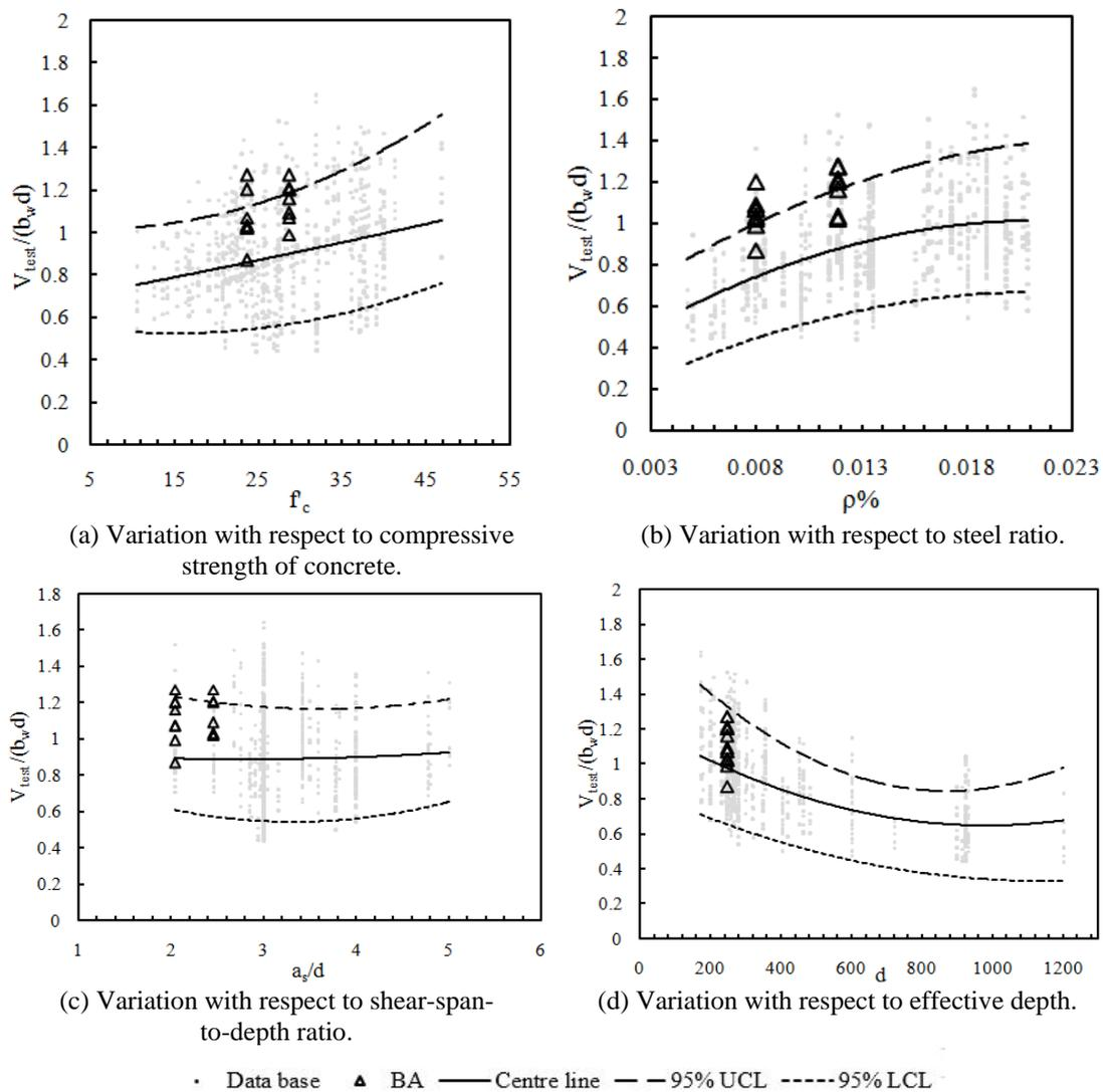
Fig. 8. Comparison of test results with shear database.
