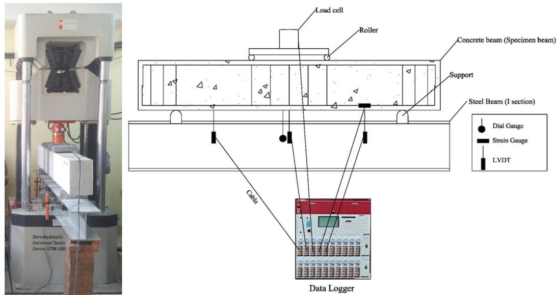
Fig. 3. Test Setup of Beams (Left – Loading in UTM Machine, Right – Connections to Data Logger).
