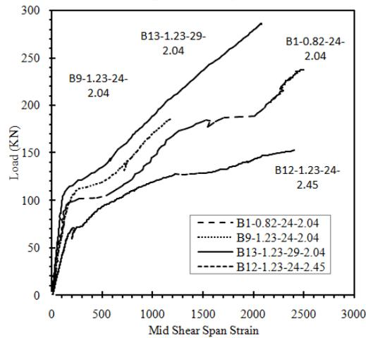
Fig. 5. Variation of strain over steel.
