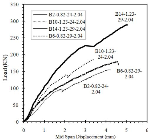
Fig. 4(a). Load-Displacement Curves of RC Beams – Shear-Span-to-Depth Ratio = 2.04
