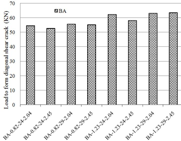
Fig. 6. Diagonal shear cracking load for BA.
