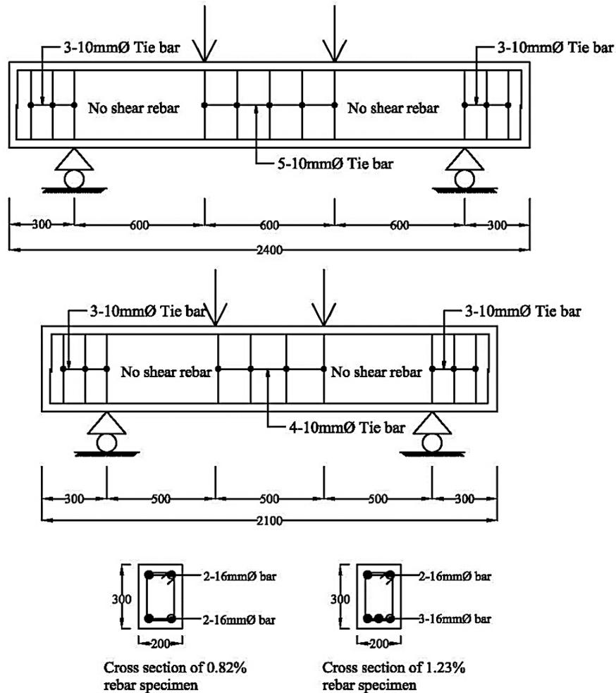
Fig. 2. Details of Reinforcement and Loading of RC Beams.
