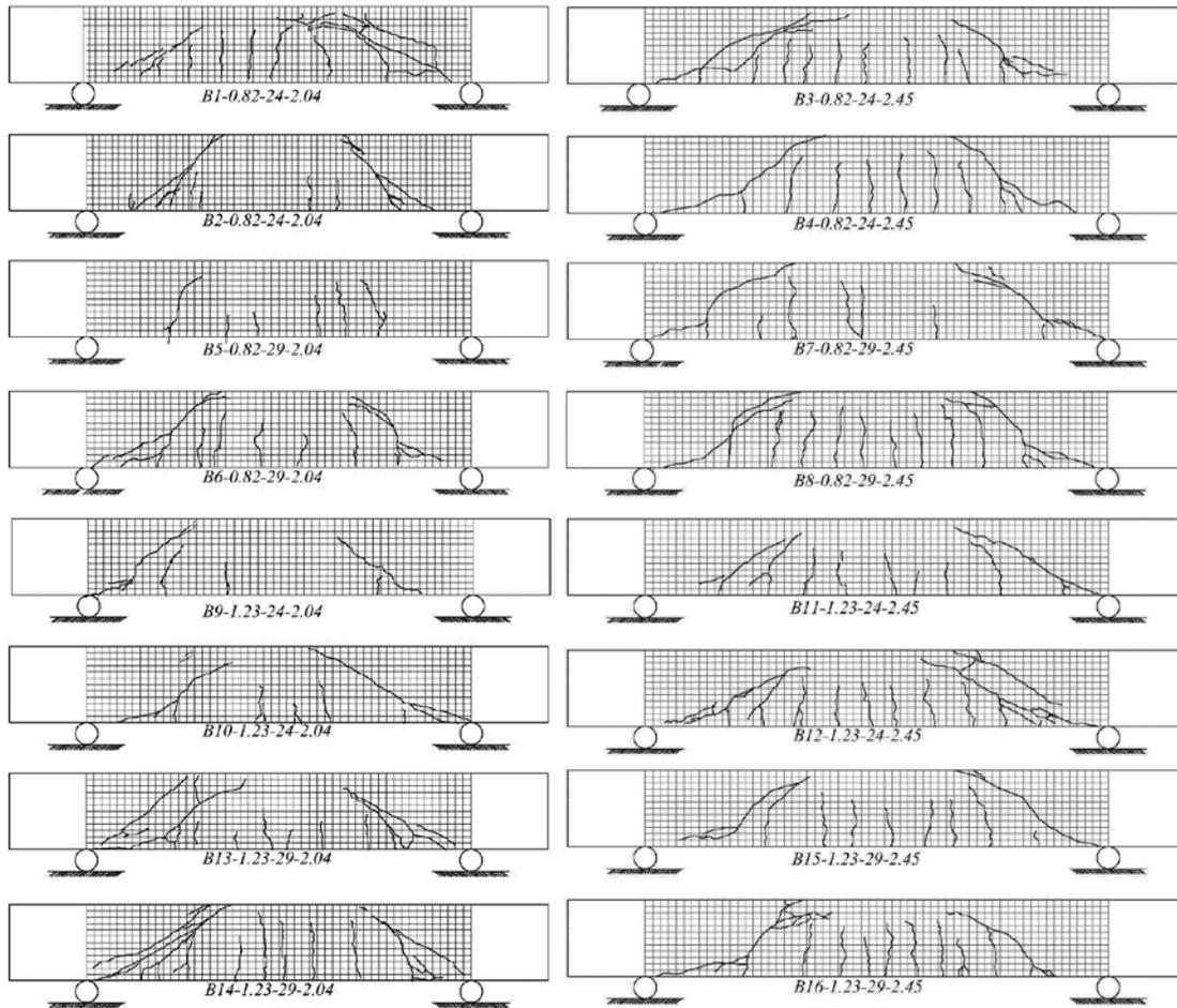
Fig. 7(a). Failure Patterns of Beams (shear-span-to-depth ratio = 2.04)
