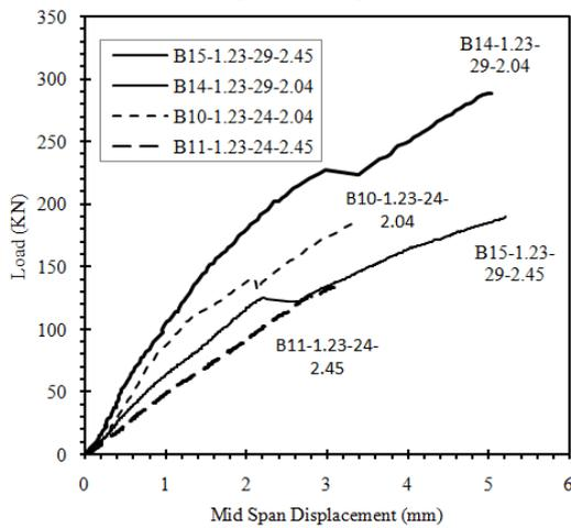
Fig. 4(c). Load-Displacement Curves of RC Beams – Steel Ratio = 1.23%
