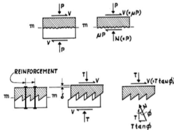
Fig. 5. Shear friction model.
