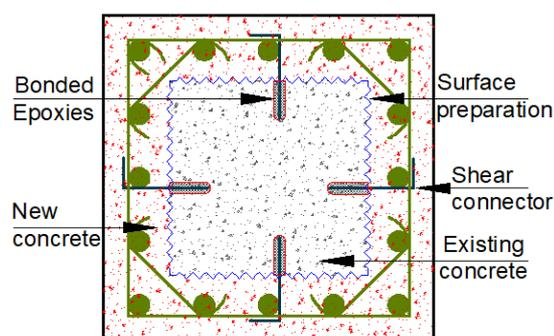
Fig. 1. Retrofitted reinforced column section.
