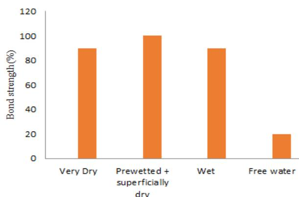
Fig. 2. Moisture condition and bond strength (Silfwerband and Beushausen, 2006).
