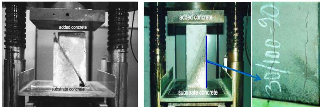
Fig. 7. a) Adhesive rupture mode of 30/30 Slant shear specimens
