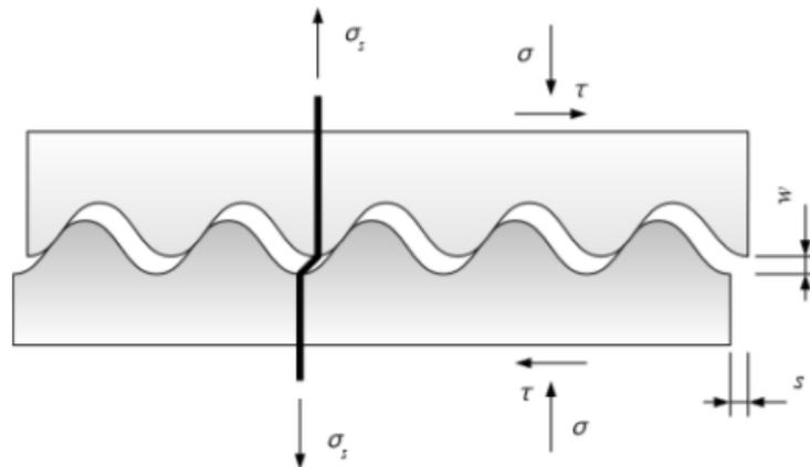
Fig. 3. Shear friction model.
