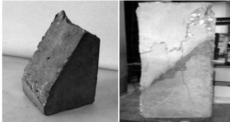
Fig. 9. Failure modes for slant shear test: (a) adhesive and (b) cohesive.
