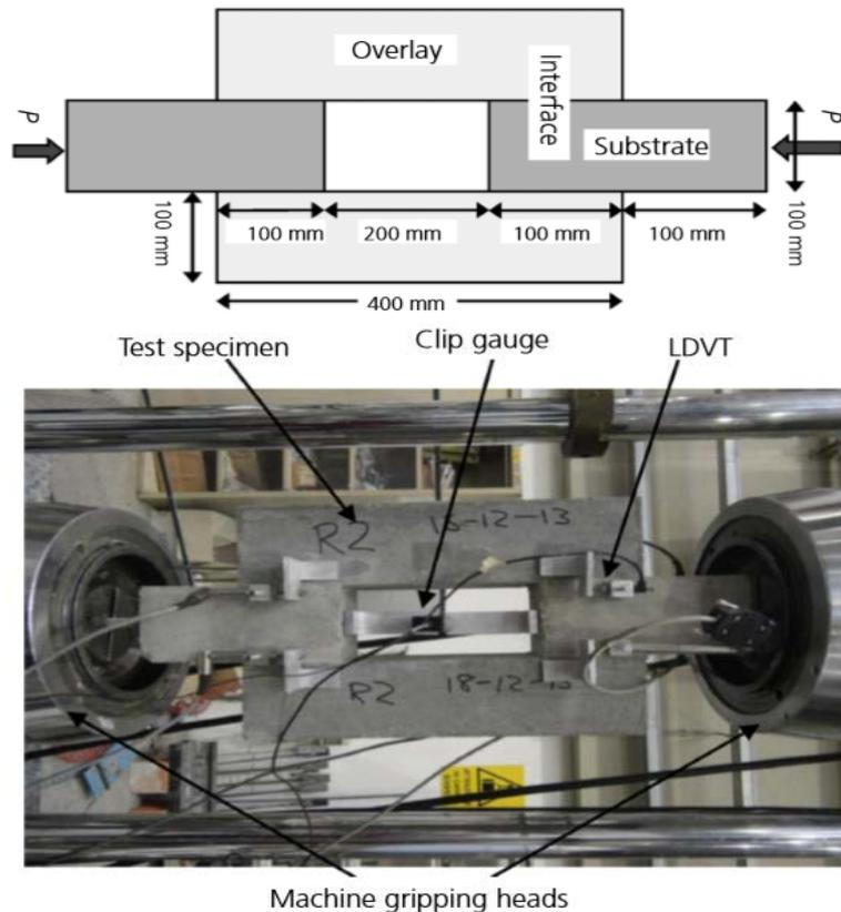
Fig. 12. Newly developed machine details.
