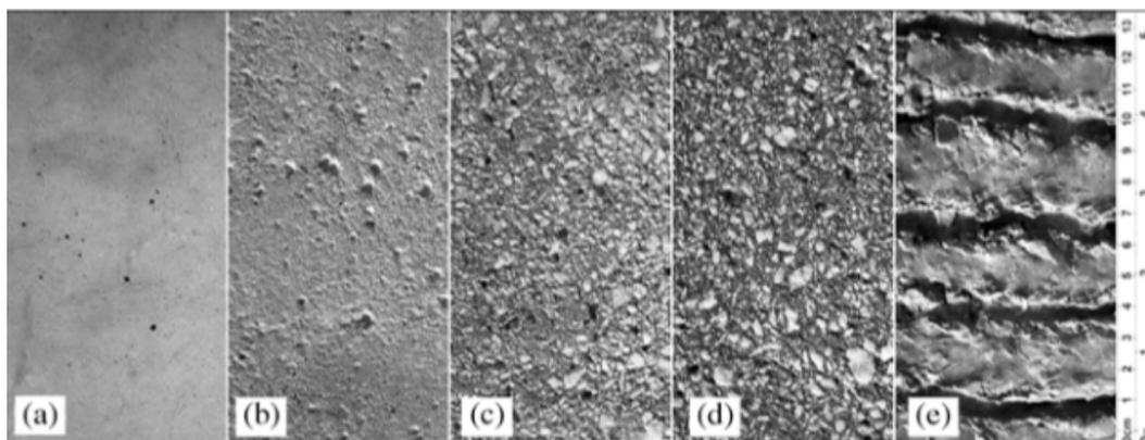
Fig. 8. Surface preparation: (a) left as-cast (b) wire-brushing (c) sand blasting (d) shot blasting and (e) hand-scrubbing(HS).
