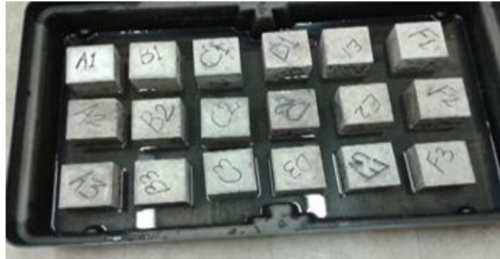
Fig. 1. Water absorption in concrete cubes
