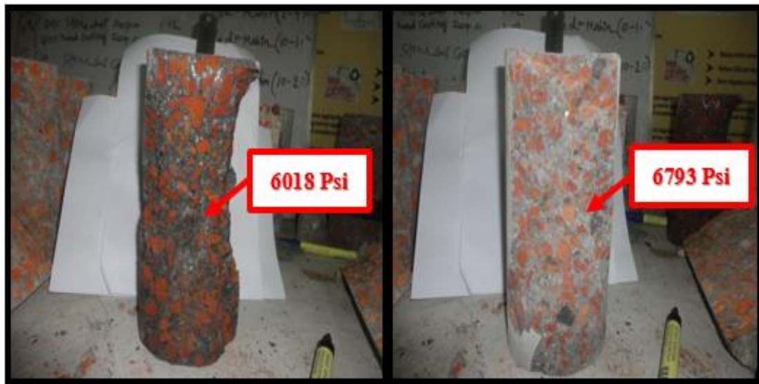
Fig. 10. Failure surfaces of concrete specimens.
