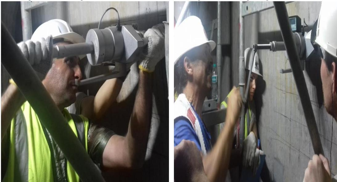
Fig. 7(a). Set-up of pull-out test instrument.
