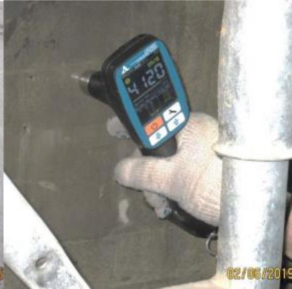
Fig. 4. Ultrasonic measurement of concrete of annular wall.
