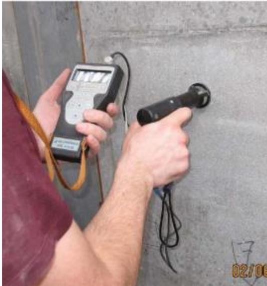
Fig. 3. Shock pulse test on annular floor walls.
