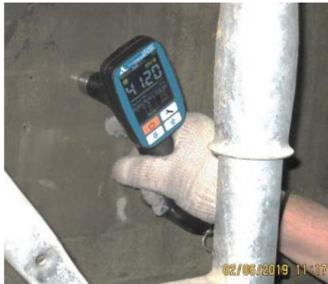
Fig. 2. Ultrasonic test on concrete annular wall.
