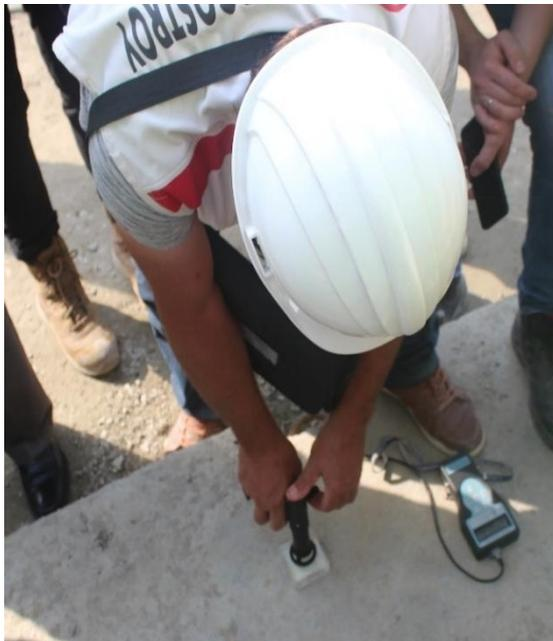
Fig. 1(a). Checking the shock impulse machine using reference block.
