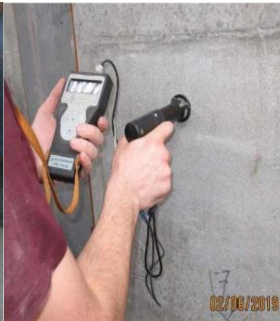
Fig. 1(b). Shock impulse test on annular floor wall.
