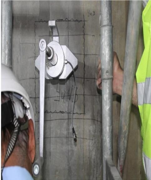
Fig. 3(a). Pull-out test on the surface.
