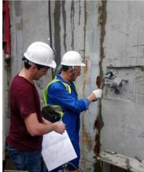
Fig. 3(b). Pull-out test at the depth of 40 mm.
