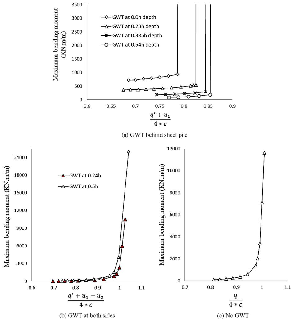
Fig. 7. Sudden large increases of maximum bending moments induced in cantilever sheet pile in terms of  $q'$ ,  $C_u$ ,  $u_1$ ,  $u_2$  in clay.
