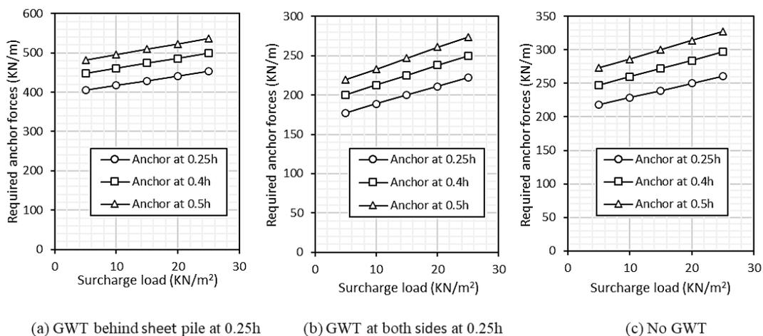
Fig. 6. Effect on anchor forces induced in single anchored sheet for lowering the position of anchor rod pile with surcharge load in sand.
