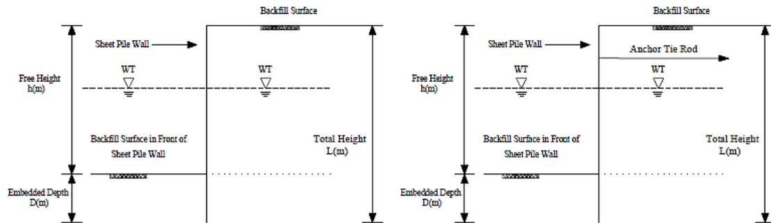
Fig. 1. Typical wall section of (a) cantilever and (b) single anchored sheet piles used in the analysis.
