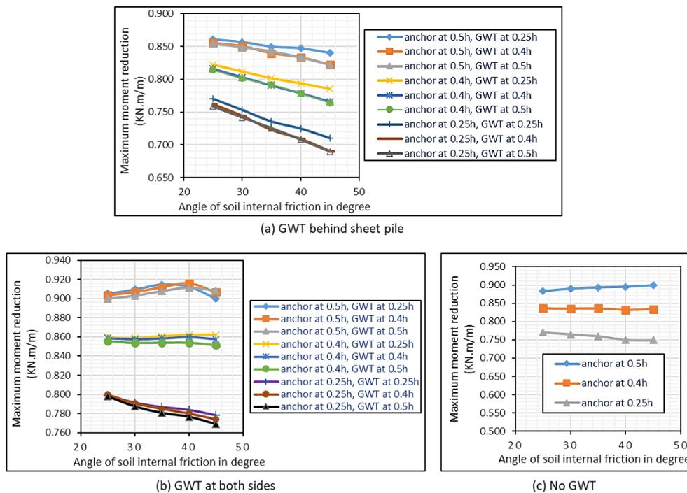
Fig. 4. Maximum bending moment reductions when using single anchor rod for different GWT conditions.
