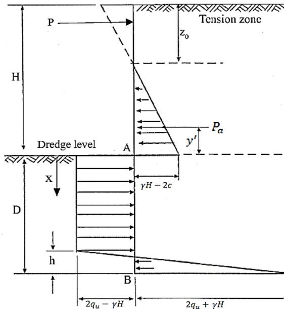
Fig. 3. Design of anchored sheet pile wall penetrating in sand without and with surcharge condition.
