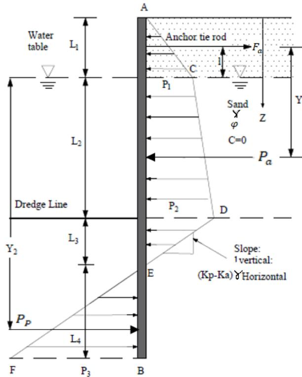
Fig. 2. Design of anchored sheet pile wall penetrating in sand without surcharge condition.
