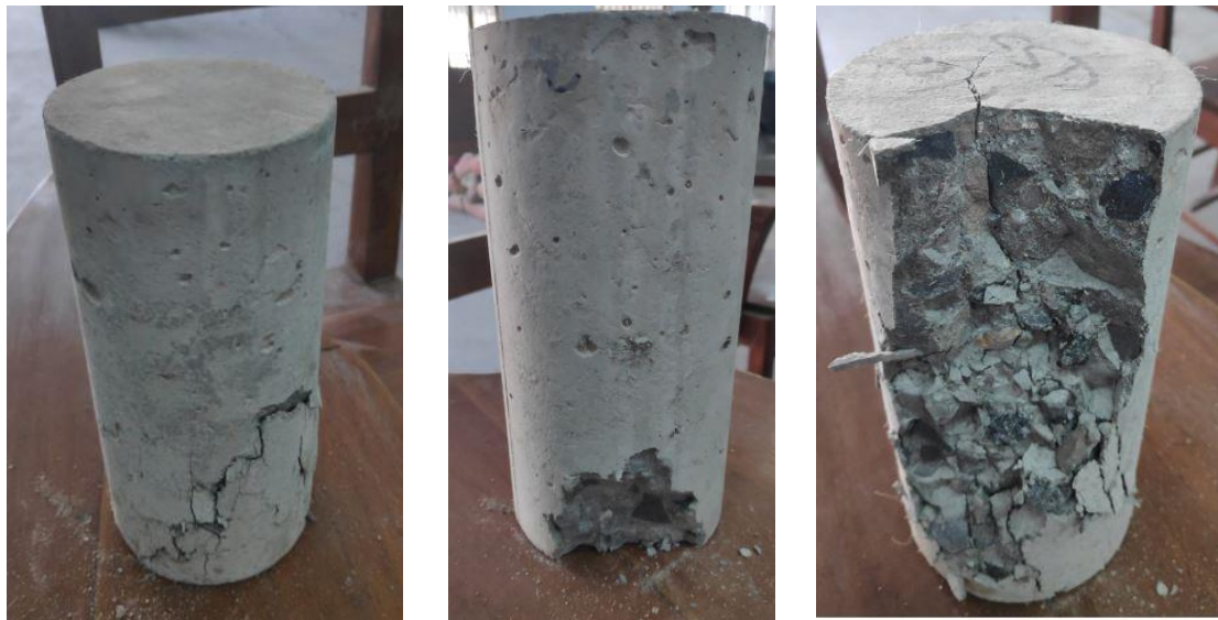
(a) (b) (c) Fig. 8. Sample control cylinders (consecutive failure types: (a) shear (b) side fracture at bottom (c) cone and shear).
