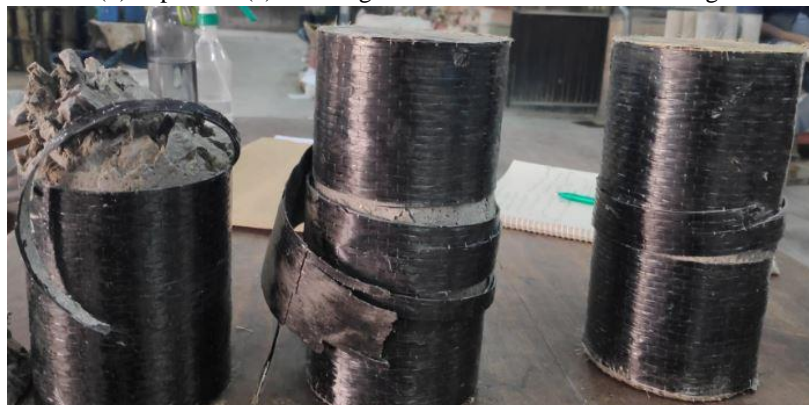
Fig. 10. Failure pattern of cylinders wrapped in three layers.
