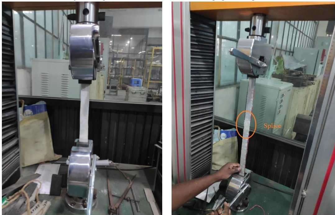
Fig. 2. Testing of flat tensile and overlap splice tension test coupons.
