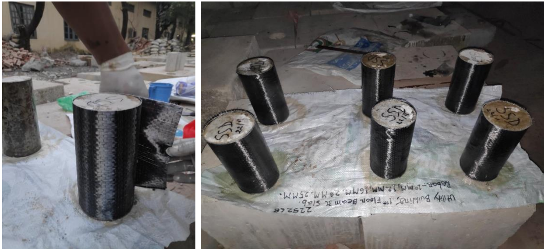
Fig. 3. CFRP Laminate wrapped cylinders ready for curing period.
