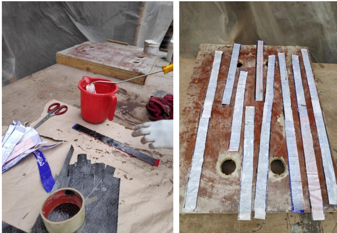
Fig. 1. Preparation of flat tensile and overlap splice coupons.
