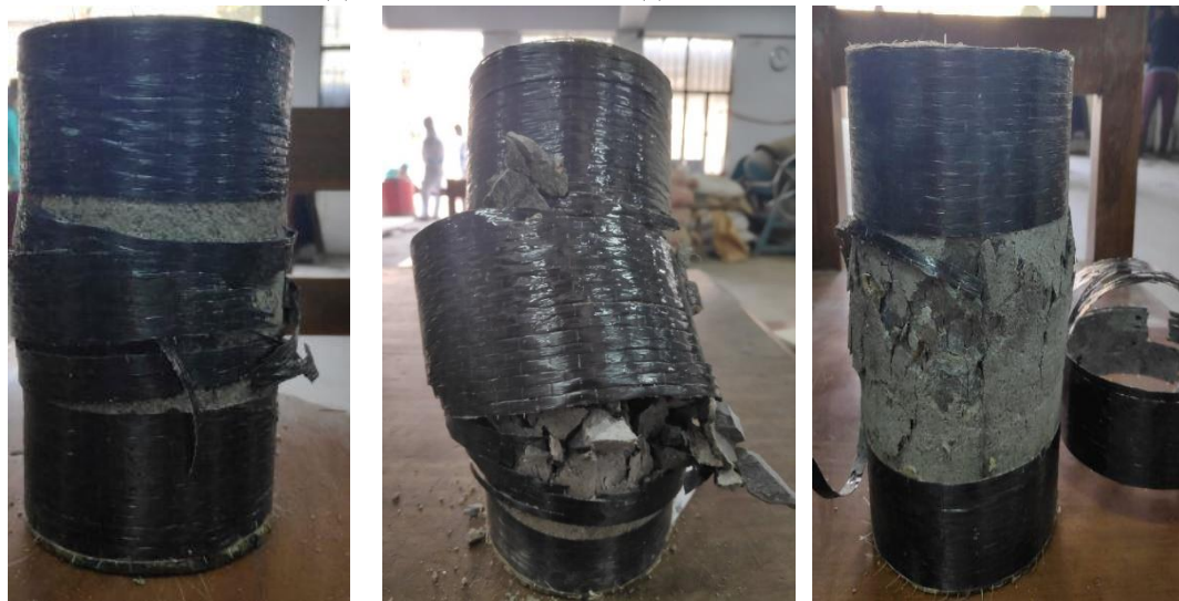
(a) (b) (c) Fig. 9. Cylinders wrapped with one layer of CFRP (a) (debonding of laminate) (b) explosive (c) crushing of concrete and fiber debonding.
