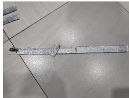
Fig. 6(b). Typical failure pattern of Overlap splice tensile coupons.
