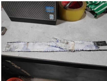
Fig. 6(a). Typical failure Pattern of Flat tensile coupons.
